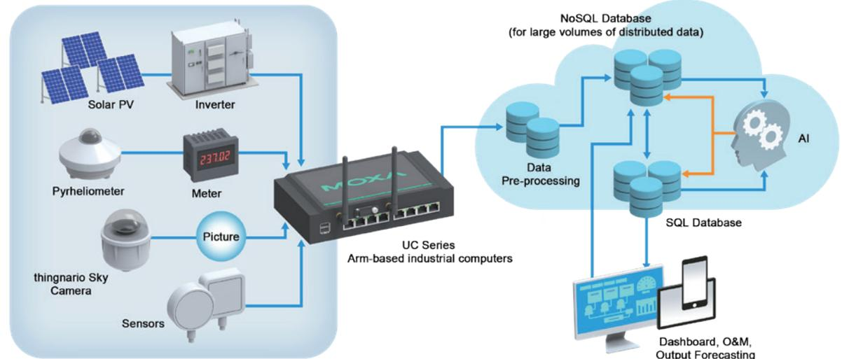
The AI engine analyzes large volumes of historical and real-time sensor data to recognize patterns and predicts how much power will be generated in the next 5 to 30 minutes.
