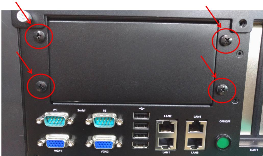
7. Install the USB Tray (with the USB dongle) and tighten the screws to secure the USB dongle tray as shown below:
