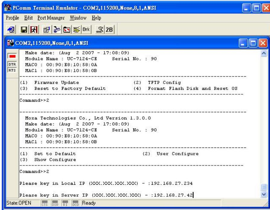
8. After providing both IP addresses, you may check the settings by typing “3” on the command line.
