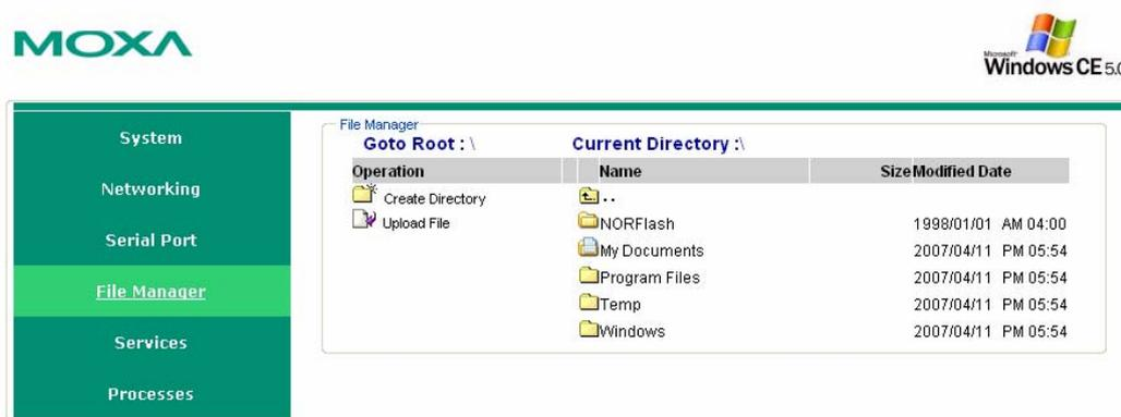
In addition, the management system offers a mechanism for uploading files. The mechanism gives you an easy way to transfer files from your workstation to the target computer. For example, after you build an application on the development workstation, you can use this mechanism to upload the application to the current directory of the target computer.
