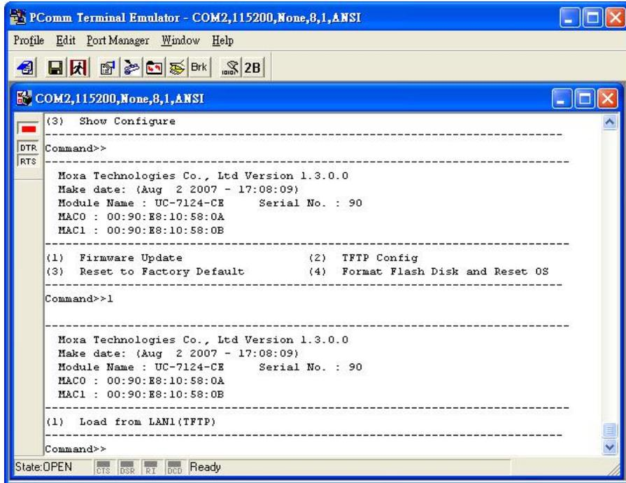
2. Type “1” to load firmware image from your PC. When prompted to provide the file name of the firmware file, input the firmware file name.
