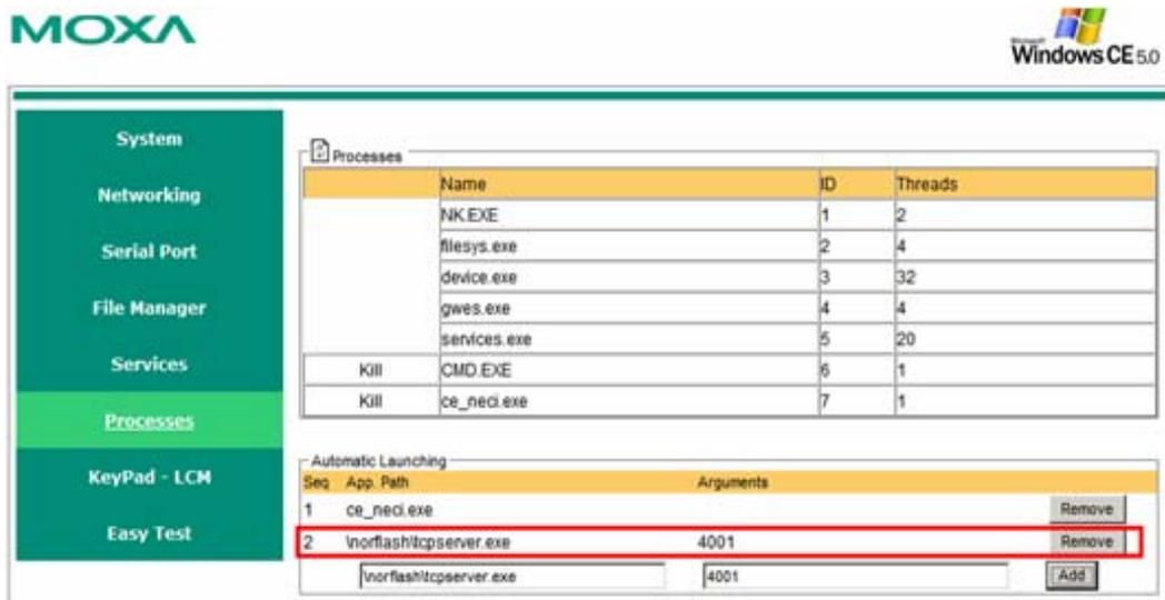
**FAQ 12** How do I monitor processes on the embedded computer?
