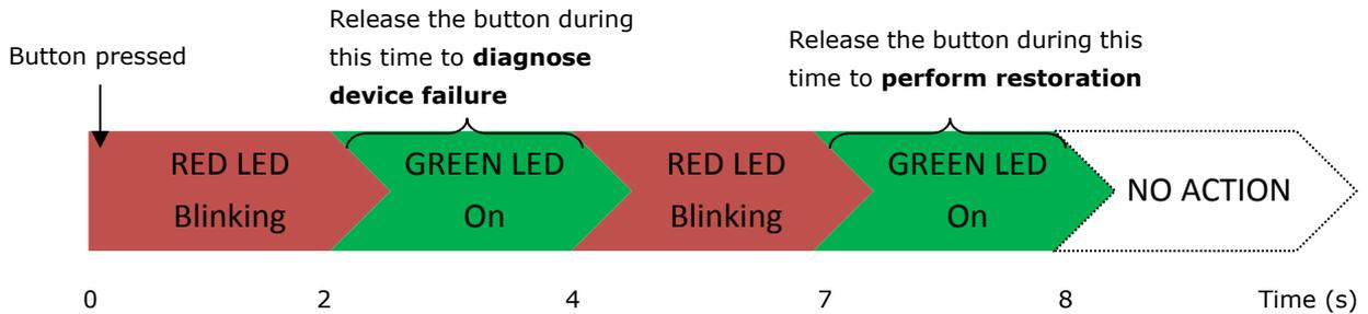
The LED indicators behave differently when diagnosing a device failure compared to performing a firmware restoration. See the following table for details.
