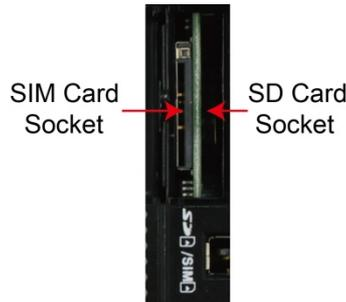
**ATTENTION** The UC-8100 does not support SD hot swap and PnP (Plug and Play) functionality. It is necessary to remove power source first before inserting or removing the SD card.
