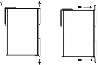
Another method for wall mounting installation is to use the optional wall mounting kit. Attach two mounting brackets on the side panel of the computer, and fasten with screws. Install the computer on a wall or cabinet by fastening two screws for each bracket.
