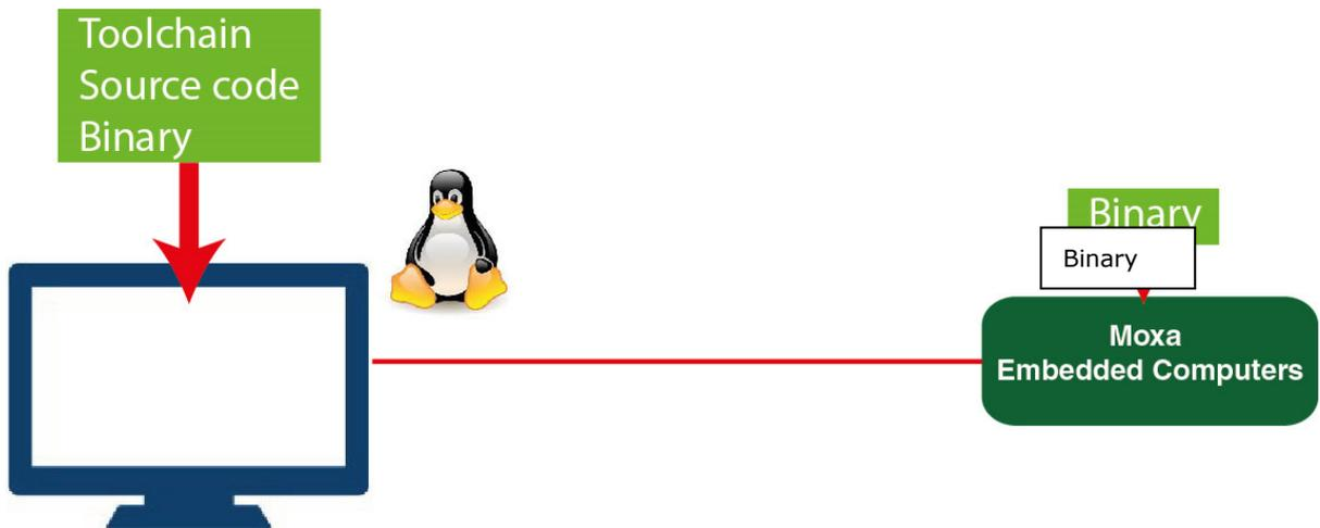
To ensure that an application will be able to run correctly when installed on the UC-8410A-LX, you must ensure that it is compiled and linked to the same libraries that will be present on the UC-8410A-LX computer. This is particularly true when the RISC Cortex processor architecture of the UC-8410A differs from the CISC x86 processor architecture of the host system, but it is also true if the processor architecture is the same.
