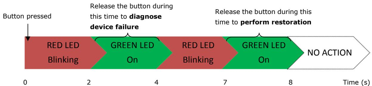
The LED indicators have different behaviors when diagnosing for device failure and for performing firmware restoration. See the following table for details.
