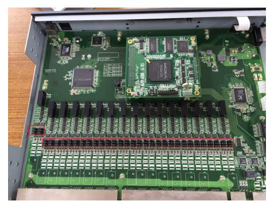
In some critical environments, you may need to add termination resistors to prevent the reflection of serial signals. When using termination resistors, it is important to set the pull high/low resistors correctly so that the electrical signal is not corrupted. The DA-662A series uses jumper settings to set the termination resistors and pull high/low resistor values for each serial port.
