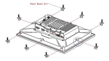
Use a torque of 4Kgf-cm to secure the mounting screws to fasten the panel-mounting kit onto the wall.
