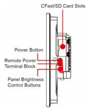
The display-control buttons can be used as described in the following table:
