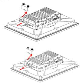
3. Reattach the cover and secure it with screws.
