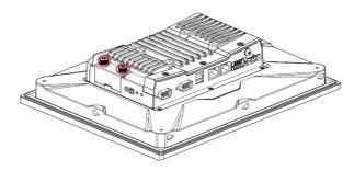
Insert the CFast or SD card into the slot using the push-push mechanism.
