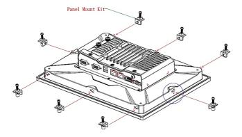
Use a torque of 4Kgf-cm to secure the mounting screws to fasten the panel-mounting kit onto the wall.
