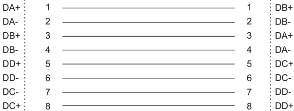
Straight-through Cable Wiring (MDI to MDI-X)
