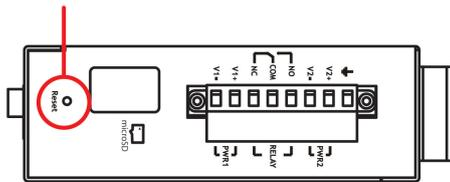
Restore the MGate to factory default settings by using a pointed object (such as a straightened paper clip) to hold the reset button down until the Ready LED stops blinking (approx. five seconds).
