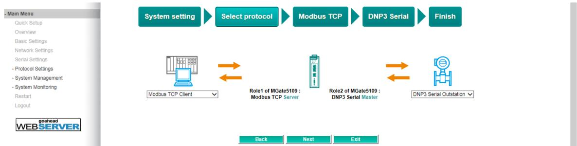
**Modbus TCP settings:** Set MGate Unit ID and TCP port.
