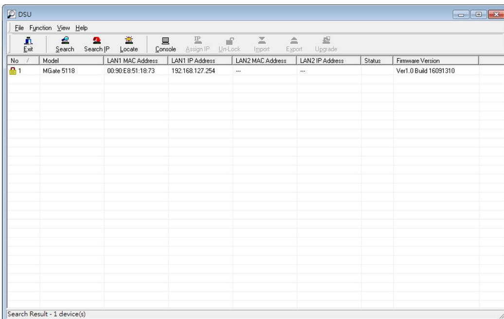
When the search is complete, every MGate 5118 found on the LAN will appear in the DSU window. The MAC address, IP address, and firmware version of each unit will be shown. Select the one you would like to configure.
