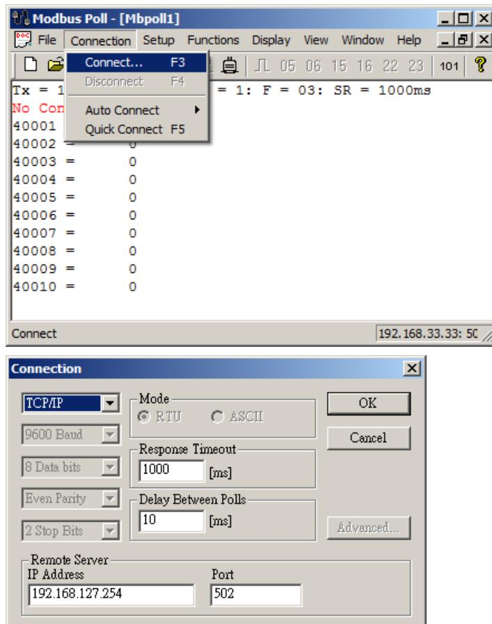
After the Modbus TCP connection is established, the application is ready.
