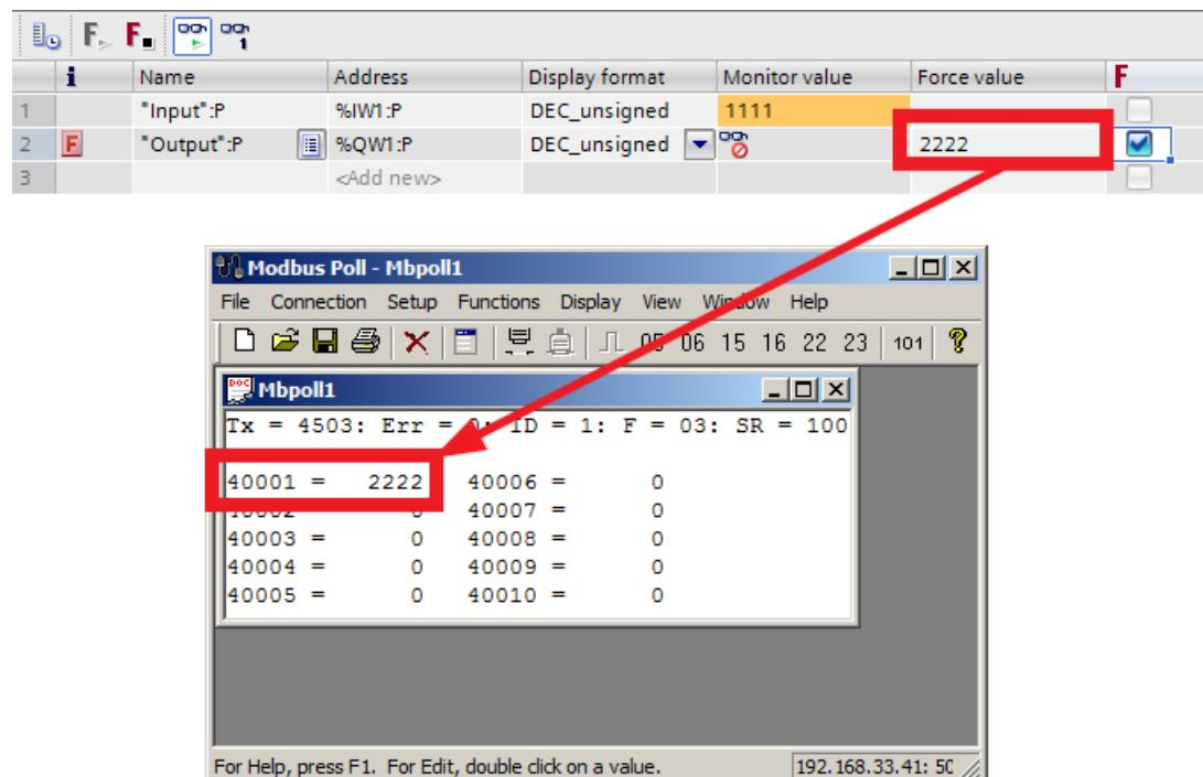
The above test confirms that the MGATE 5101-PBM-MN will poll the PROFIBUS slave device regularly.
