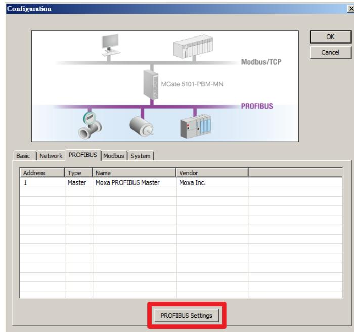
6.2.4. Select **PROFIBUS → AutoScan** or click the **AutoScan** button to enable the AutoScan function to scan the PROFIBUS slave device automatically.
