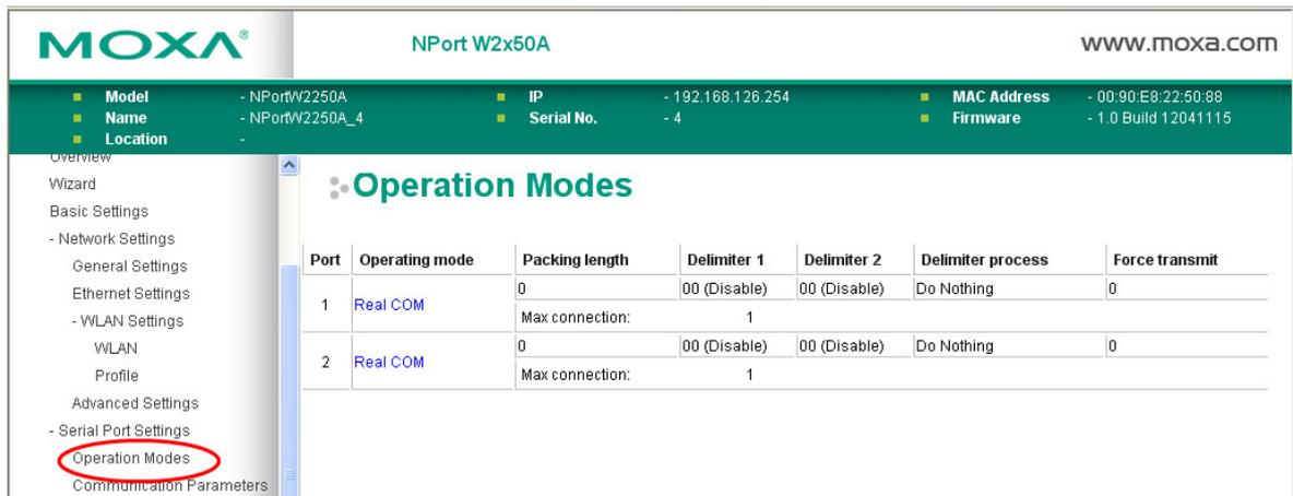
Each serial port on the NPort is configured through the hyperlink below the column of **Operating mode**.
