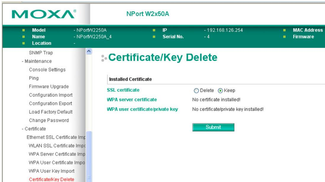
The **Certificate/Key Delete** page is located under **Certificate** in the **System Management** folder. This page is where you can delete certificates or WPA keys that have been installed on the model. When you click **[Submit]**, any certificate or key that has been set to **Delete** will be deleted from the NPort.
