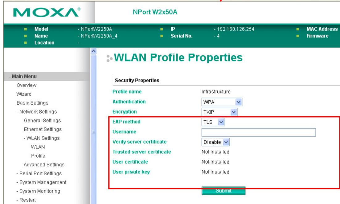
When WPA or WPA2 is used for authentication, you will also need to configure **EAP method** in the **Security** settings for the WLAN profile. Other settings will also be displayed depending on how **EAP method** is configured.
