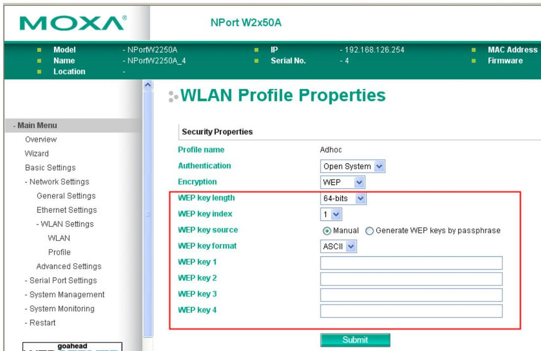
When Encryption is set to WEP on the **Security** page for the WLAN profile, you will be able to configure **WEP key length**, **WEP key index**, and **WEP key source**. Other settings will be displayed depending on how **WEP key source** is configured.
