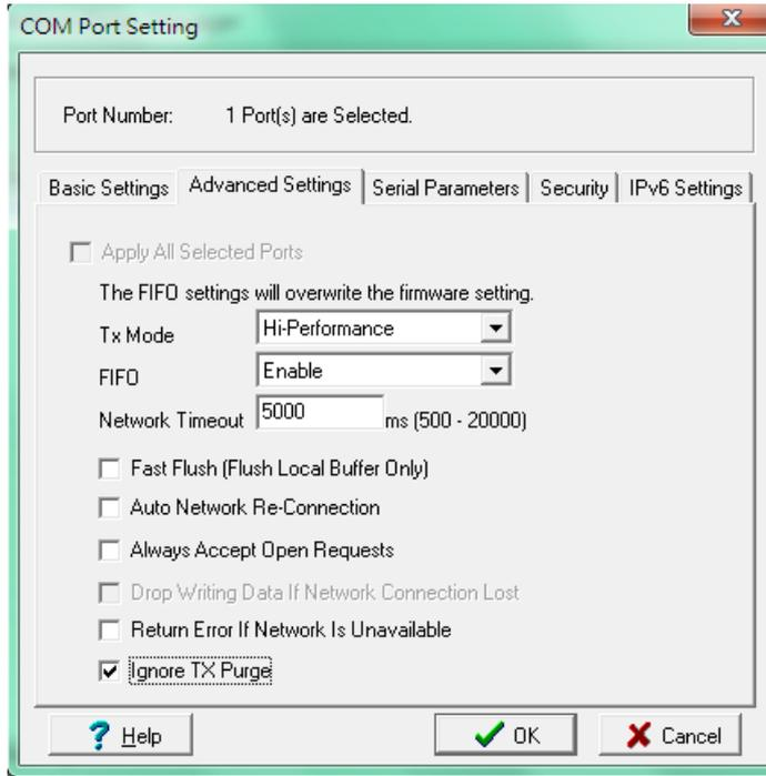
**Tx Mode:** In Hi-Performance mode, the driver immediately issues a "Tx Empty" response to the program after sending data to the NPort. In Classical mode, the driver sends the "Tx Empty" response after confirmation is received from the NPort. Classical mode is recommended if you want to ensure that all data is sent out before further processing.
