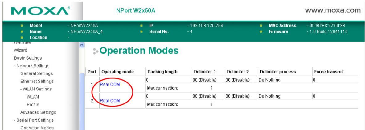
Click the link of **Real COM**, it will show the Port settings page. The Operation Modes page for each serial port is where you configure the serial port's operation mode and related settings. For an introduction to the different operation modes, please refer to Chapter 4.
