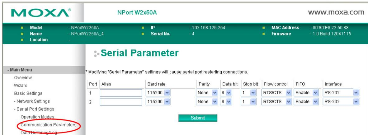
The **Communication Parameters** page for each serial port is where serial communication settings are specified, such as **Baud rate**, **Data bits**, and **Stop bits**.
