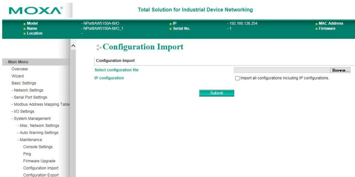
The **Configuration Import** page is located under **Maintenance** in the **System Management** folder. This is where you can load a previously saved or exported configuration. Select or browse for the configuration file in the **Select configuration file** field. If you also wish to import the IP configuration (i.e., IP address, netmask, and gateway), make sure that **Import all configurations including IP configurations** is checked.
