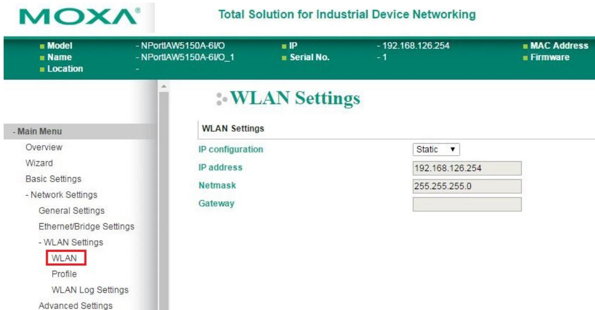
The **WLAN** page is located under **WLAN Settings** in the **Network Settings** folder. You can modify **IP configuration**, **IP address**, **Netmask**, and **Gateway** for your WLAN.
