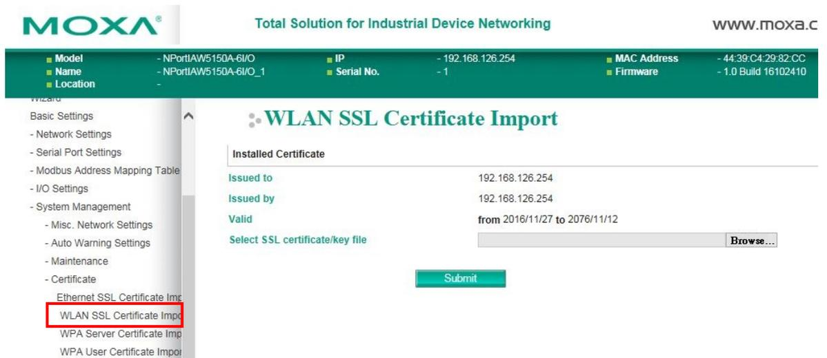
The **WLAN SSL Certificate Import** page is located under **Certificate** in the **System Management** folder. By default, the WLAN SSL certificate is automatically generated by the NPort based on the IP address of the wireless interface. You can also import a certificate. Select or browse for the certificate file in the **Select SSL certificate/key file** field.
