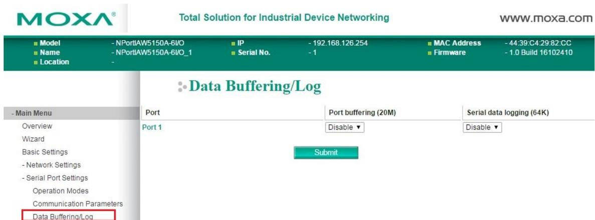
On the serial port's **Data Buffering/Log** page, you can enable or disable **Port buffering** and **Serial data logging**.
