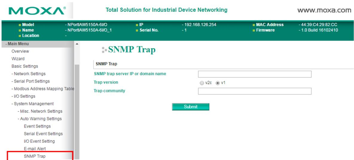
The **SNMP Trap** page is located under **Auto Warning Settings** in the **System Management** folder. This is where you specify the SNMP trap settings to use for automatic notification of system and serial port events.
