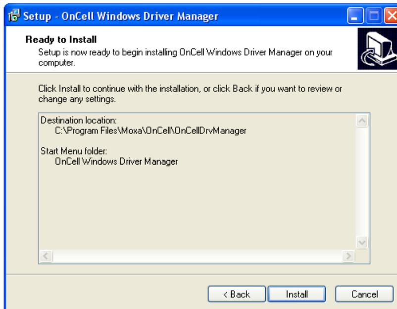
5. Click **Install** to begin the installation. The setup window will report the progress of the installation. To change the installation settings, click **Back** and navigate to the previous screen. On Windows XP, the installer will display a message that the software has not passed Windows Logo testing. This is shown as follows:
