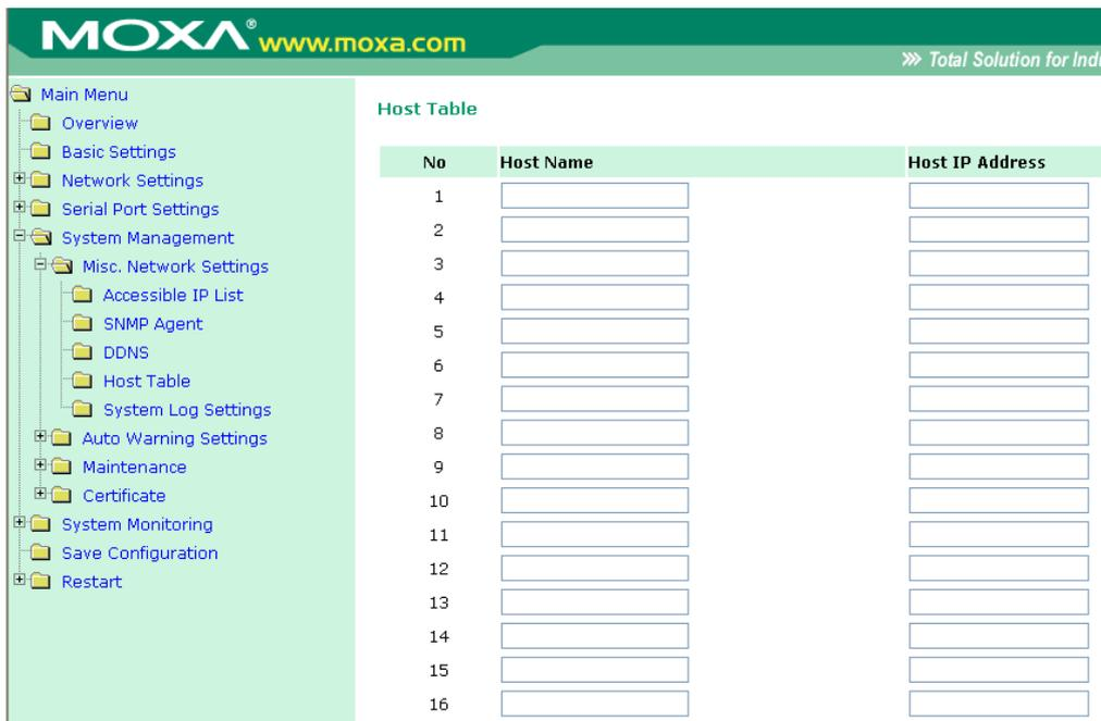
The Host Table can be used to simplify IP address entry in the OnCell G3111/G3151/G3211/G3251 console by assigning a Host Name to a Host IP Address. When you assign a Host Name to a Host IP Address, you can then use the Host Name for some fields on the console rather than entering the IP address. Up to 16 entries can be stored in the Host Table.
