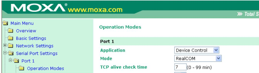
Select **Operation Modes** in the navigation panel to select and configure the mode for each serial port.
