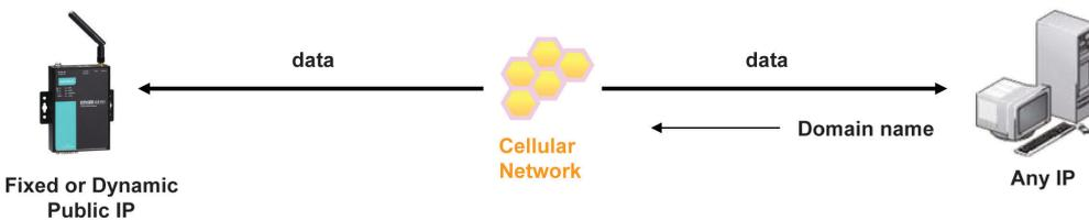
4. Connecting TCP client and TCP server within the same cellular service provider.
