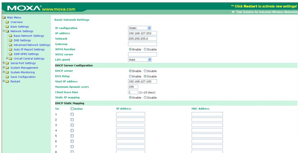
You can access **Basic Network Settings** by expanding the **Network Settings** item in the navigation panel. Basic Network Settings is where you assign the OnCell G3111/G3151/G3211/G3251's IP address, netmask, Gateway, and other parameters for the Ethernet interface.
