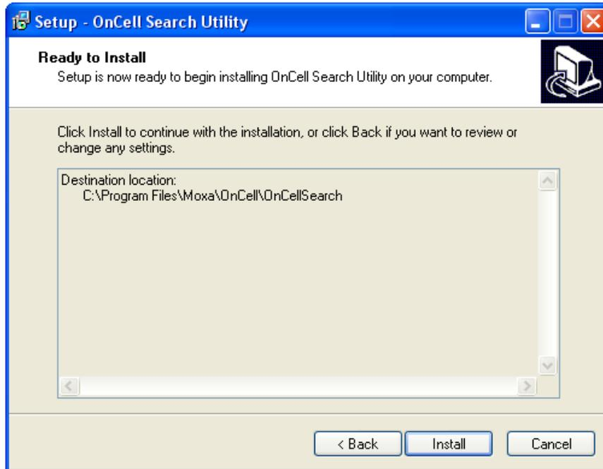
6. Click **Install** to begin the installation. The setup window will report the progress of the installation. To change the installation settings, click **Back** and navigate to the previous screen.
