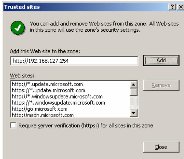
After adding the OnCell G3111/G3151/G3211/G3251’s IP address as a trusted site, you should be able to view the web console by entering the OnCell G3111/G3151/G3211/G3251’s IP address in your browser’s address bar.
