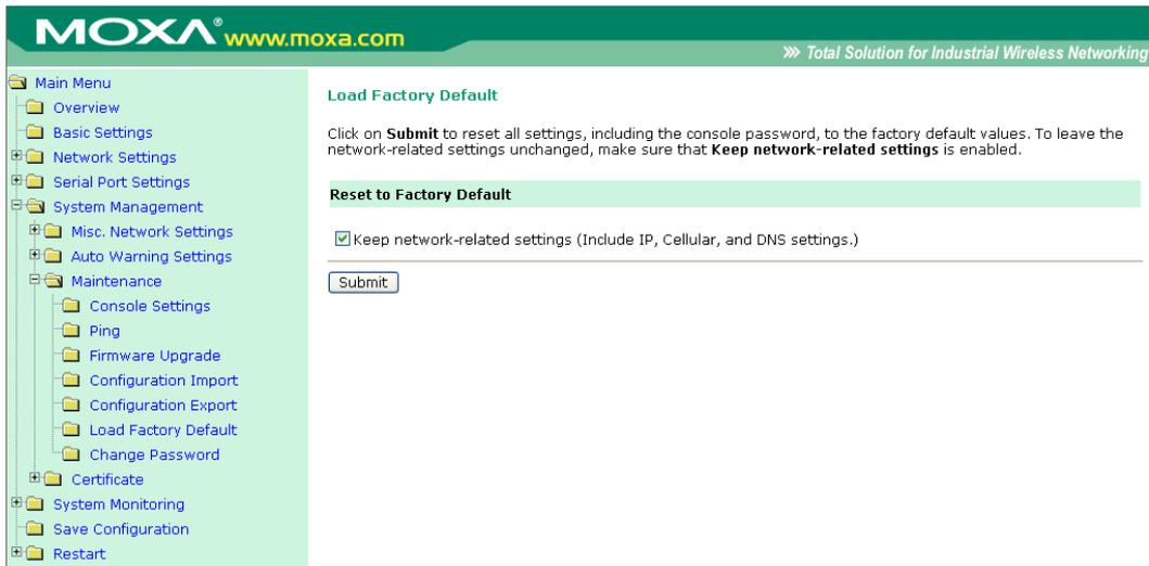
This function will reset all of OnCell G3111/G3151/G3211/G3251's settings to the factory default values. All previous settings including the console password will be lost. If you wish to keep the OnCell G3111/G3151/G3211/G3251 IP address, netmask, and other IP settings, make sure **Keep IP settings** is checked off before loading the factory defaults.
