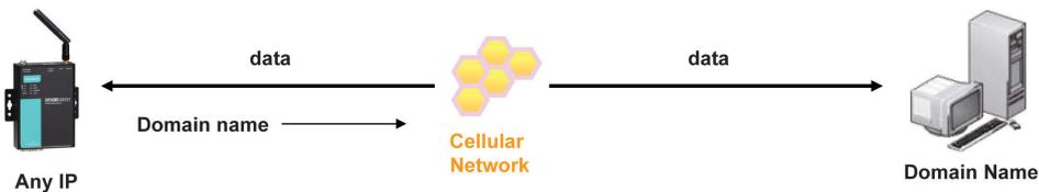
3. Connecting TCP client and TCP server within the same cellular service provider.
