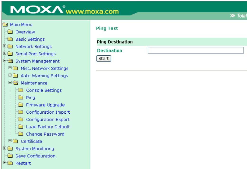
You can ping an IP address from the OnCell G3111/G3151/G3211/G3251 web console in order to test the Ethernet connection. Enter the IP address or domain name in the **Destination** field to make sure that the connection is OK.
