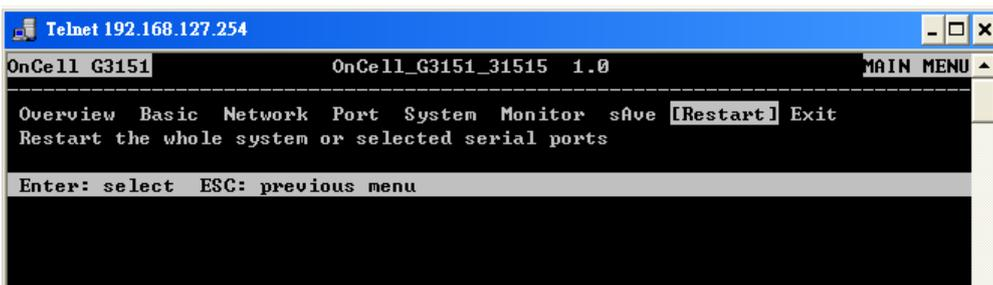
11. Press **S** or use the arrow keys to select **System** and then press **ENTER** to restart the OnCell G3111/G3151/G3211/G3251.
