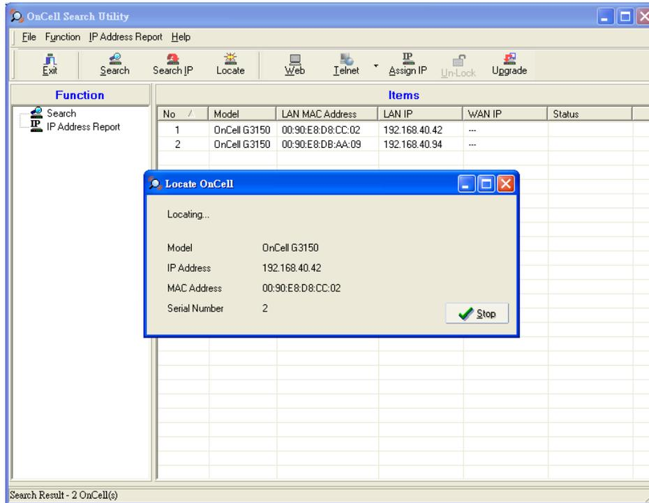
To modify the configuration of the highlighted OnCell G3111/G3151/G3211/G3251, click on the Console icon to open the web console. This will take you to the web console, where you can make all configuration changes. Refer to **Chapter 5, Using the Web Console**, for information on how to use the web console.
