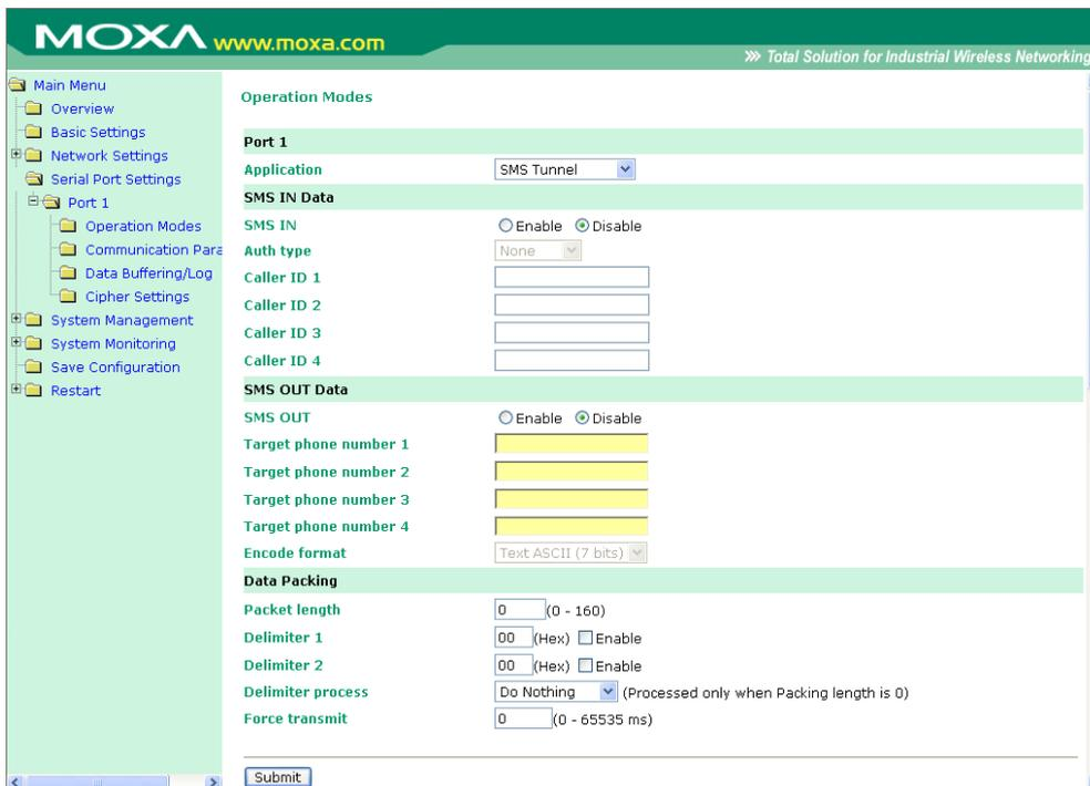
**SMS IN enable (default = Disable):** To allow forwarding incoming short message to the OnCell G3111/G3151/G3211/G3251's serial port as data.
