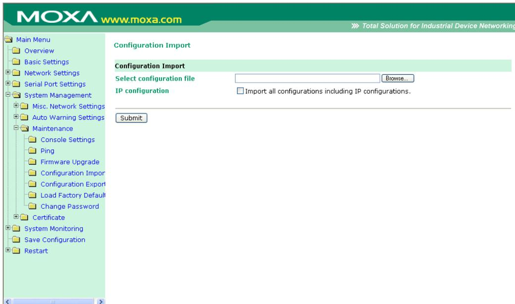
To import a configuration, go to **System Management** → **Maintenance** → **Configuration Import**. Enter the configuration file path/name and click **Submit**. The OnCell G3111/G3151/G3211/G3251's configuration settings will be updated according to the configuration file. If you also wish to import the IP configuration (i.e., the OnCell G3111/G3151/G3211/G3251's IP address, netmask, gateway, etc.), make sure that **Import all configurations including IP configurations** is checked on.
