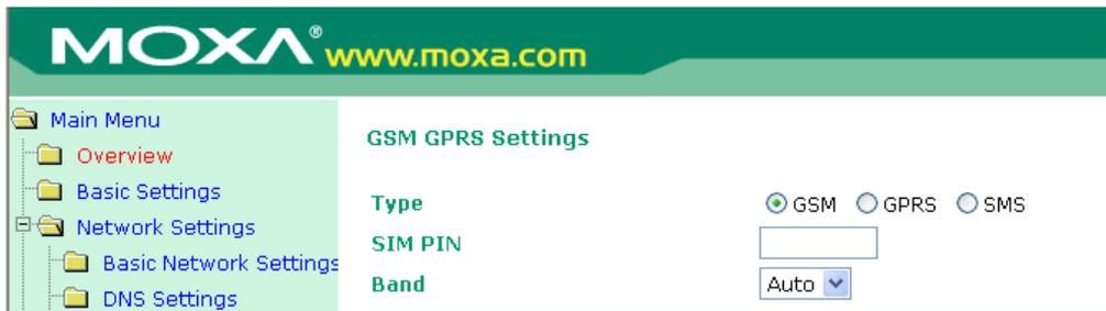
From the left navigation panel, click **Network Settings → GSM GPRS Settings** to configure the GSM/GPRS/SMS Settings. The various configuration items are described below:
