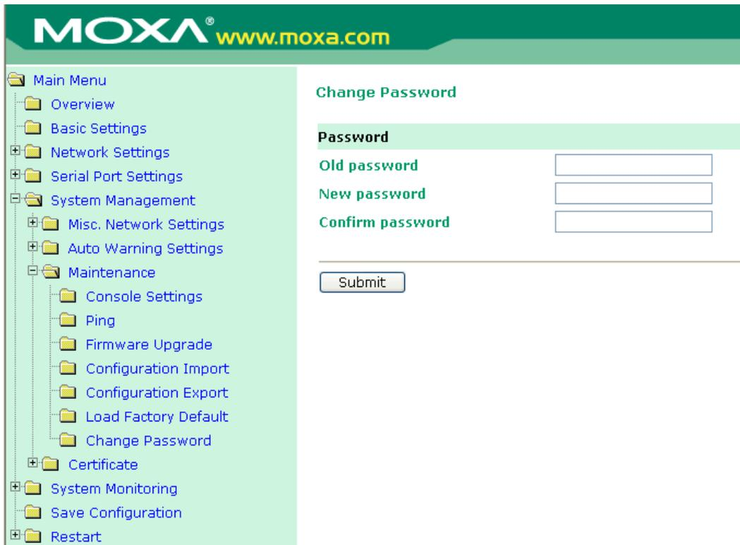
For all changes to the OnCell G3111/G3151/G3211/G3251's password protection settings, you will first need to enter the old password. Leave this blank if you are setting up password protection for the first time. To set up a new password or change the existing password, enter your desired password under both **New password** and **Confirm password**. To remove password protection, leave the **New password** and **Confirm password** boxes blank.
