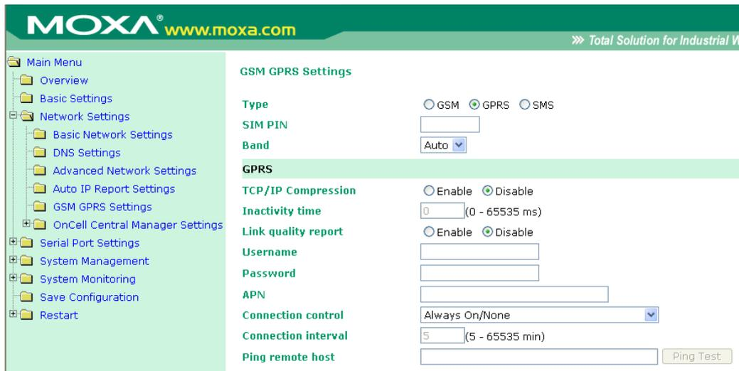
**TCP/IP compression (default=Disable):** The setting of this field depend on whether or not the remote user's application requests compression.
