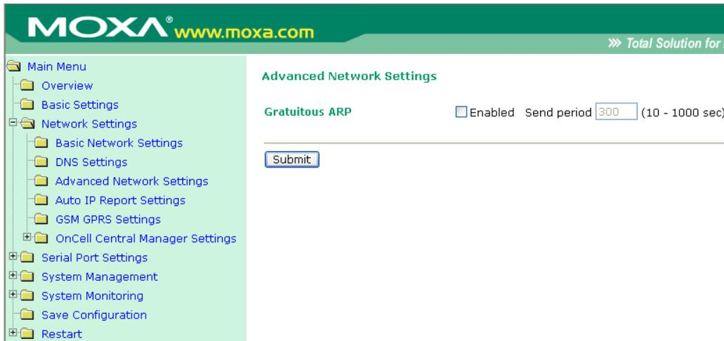
**Gratuitous ARP:** In some applications, you may need the OnCell G3111/G3151/G3211/G3251 to send broadcast packets to update the ARP table on the server. If you enable this function and set the send period, the OnCell G3111/G3151/G3211/G3251 will periodically send broadcast packets at the specified time interval.
