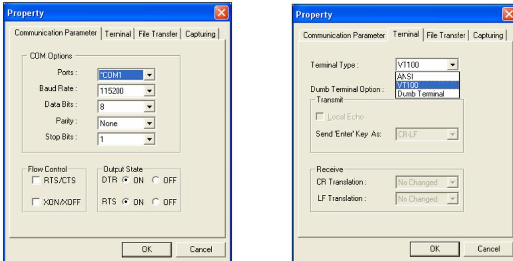
The Communication Parameter page of the Property window will appear. Select the appropriate COM port for Console Connection, 115200 for Baud Rate, 8 for Data Bits, None for Parity, and 1 for Stop Bits
