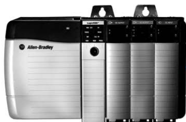
Allen-Bradley PLC IP: 192.168.108.200
