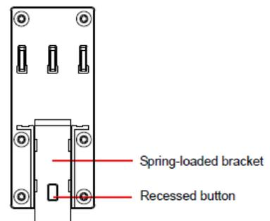
**STEP 2:** Insert the top of the DIN-Rail into the top slots on the DIN-Rail attachment plate.
