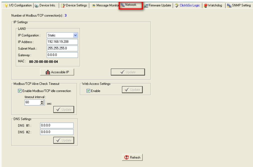
**IP Settings:** You can set up a static or dynamic IP address for both of the ioPAC 8020 LAN ports, as well as the subnet mask and gateway address.
