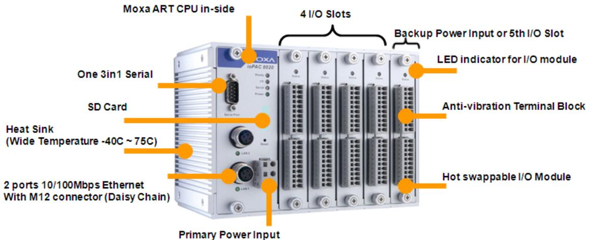
The ioPAC modular RTU controller consists of two major components: the CPU Module, which includes empty I/O slots, and the I/O modules themselves. The CPU module provides the capability for daisy-chain communications over Ethernet networks, includes simple logic control, and powers the whole system. Each CPU module is equipped with five I/O slots for different I/O modules. The last module slot can be filled by a backup power module or an additional I/O module.
