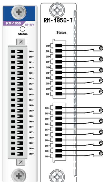
**RM-1050-T: 10 digital inputs, 110 VDC, isolated**
