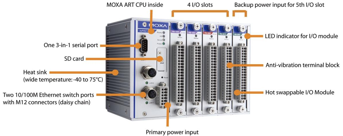
The ioPAC 8020 uses 24 VDC power inputs. One power input is required, and a second one can be used as a backup power input. The ioPAC 8020 provides 5 VDC power to all connected I/O modules. When the total current consumption of the I/O modules exceeds 1.5A, you will need to insert an extra power module.
