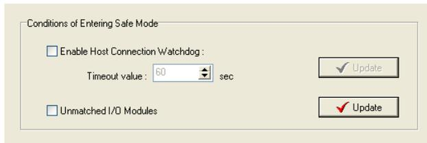
After **one of these two conditions** is enabled, the ioPAC 8020 will enter safe status. Click the Watchdog Tab to exit safe status. The system will display the message **Host Connection Lost Alarm or I/O Error**, indicating that the system is in safe status. Click Clear Alarm to exit safe status and return to normal operation manually.
