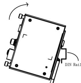
**STEP 3:** The DIN-Rail attachment unit will snap into place as shown in the illustration to the right.
