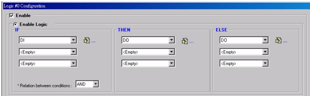
Click&Go Logic was developed to provide an easy and intuitive way to configure when and how I/O information is transmitted over the network. Using simple IF-Then-Else statements, you set the conditions that need to be satisfied and the resulting actions. Up to three conditions and three actions can be combined in any one rule, and up to 80 rules can be defined in a ruleset. Each SNMP trap, TCP/UDP message can be transmitted to up to 10 hosts simultaneously.
