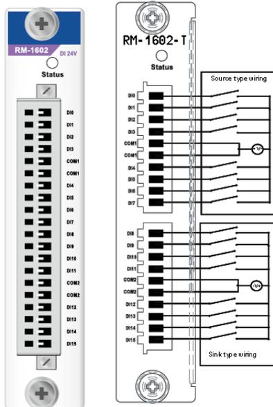
**RM-1602-T: 16 digital inputs, 24 VDC, sink/source type**
