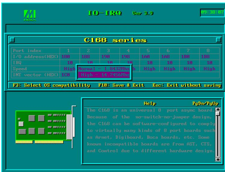
Note that, currently, port that uses **MOXA Windows NT and 95/98 driver** will run at the displayed speed. To be clear, when Smartio C168 Series board is configured as **High Speed Spectrum**, any port driven by the **Moxa-provided Windows NT and 95/98 driver** will display the exact working speed. For example, the displayed speed 38.4 Kbps is equal to the working speed 38.4 Kbps.
