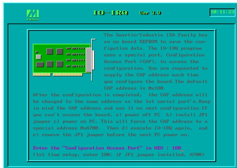
3. Enter the CAP address of the Smartio C168 Series board to be configured.
