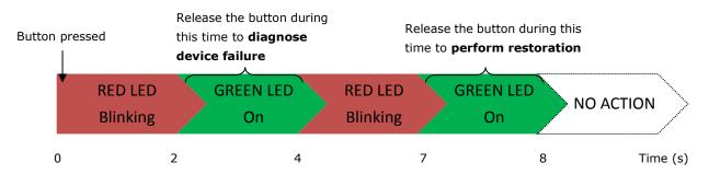
The LED indicators have different behaviors when diagnosing for device failure and for performing firmware restoration as listed in the table below:
