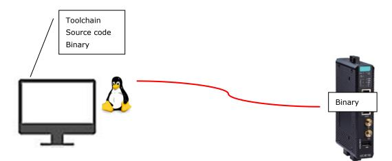
To ensure that an application will be able to run correctly when installed on the UC-8100-LX, you must ensure that it is compiled and linked to the same libraries that will be present on the UC-8100-LX computer. This is particularly true when the RISC Cortex processor architecture of the UC-8100 differs from the CISC x86 processor architecture of the host system, but it is also true if the processor architecture is the same.
