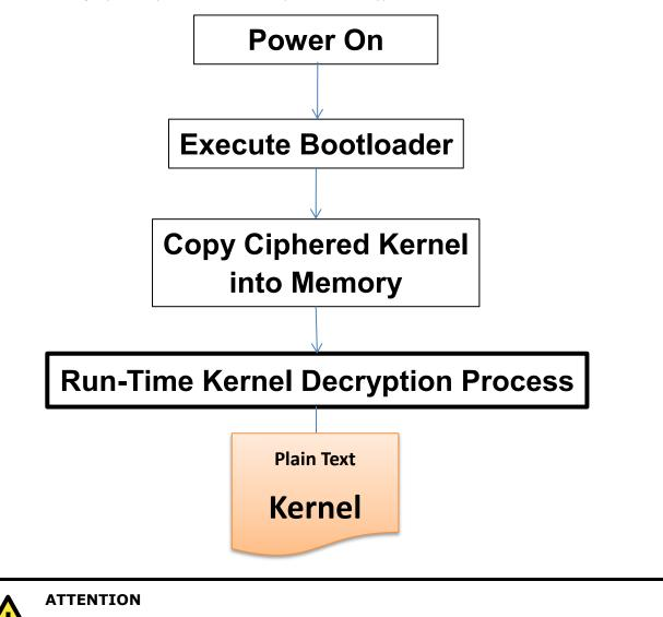
Do NOT arbitrarily replace the kernel or bootloader, or the computer will not be able to boot up.
