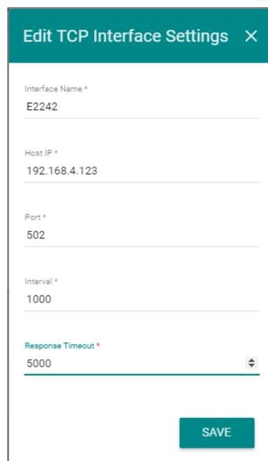
The Modbus/TCP interface for E2242 is added to the **TCP List**.
