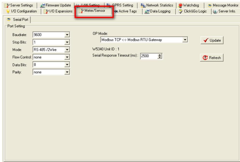
**Step 3:** Set the serial port parameters: RS-232, RS-485, Baudrate, Stop Bits, etc.
