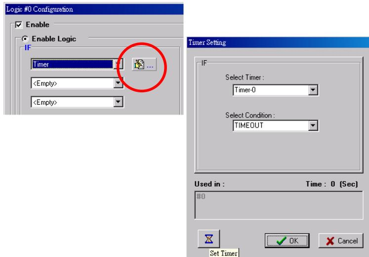
In the above figure, the "Used in:" column indicates this Timer is also used in Rule-0, which helps the user identify the relationship between rules. In addition, the Set Timer button (
