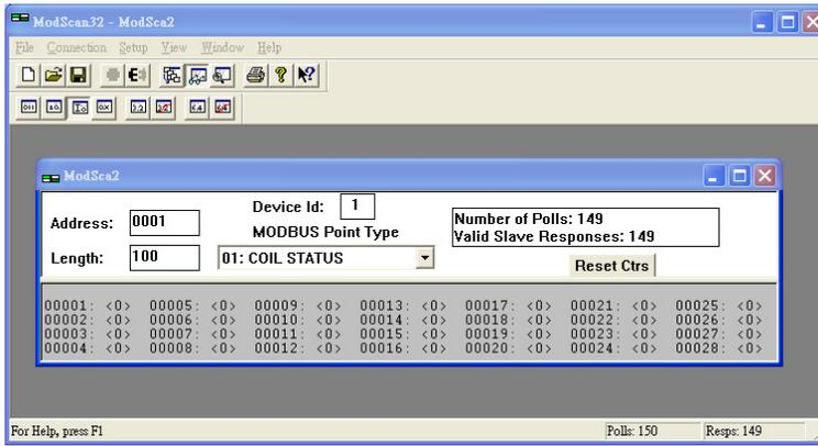
**Step 10:** Look up the DI-0 and DI-1 Modbus addresses in the user’s manual, as shown below.
