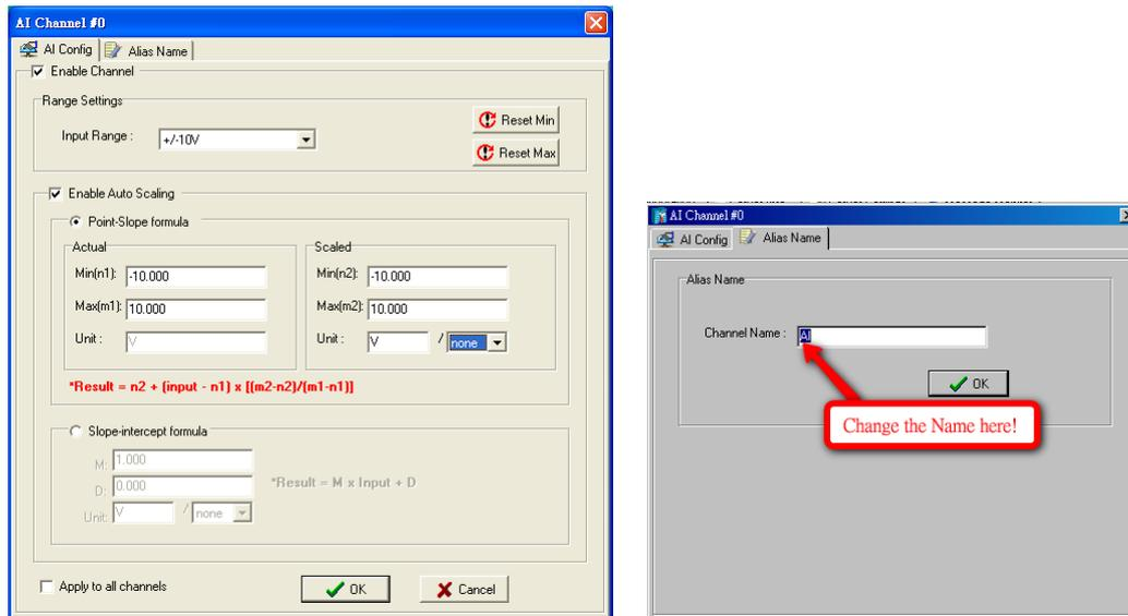
Users can disable the unused AI channel by un-checking the **Enable** check box to increase the sampling rate.
