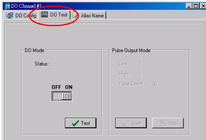
After clicking the Test tab, you can see how a channel's status affects or is affected by the attached device. For DO channels, you can set the on/off status or start and stop pulse output. For DI channels, you can monitor the attached device's on/off status, or monitor the counter.
