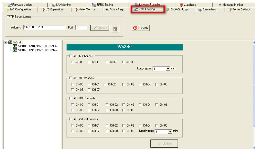
**Step 3:** Input the TFTP IP address.
