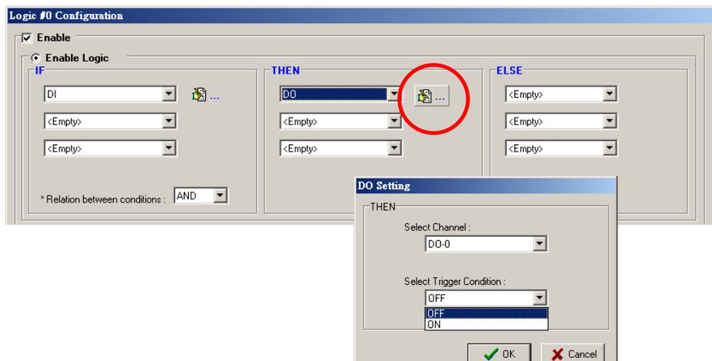
**NOTE** A Relay output channel is also referred to as a DO channel in the THEN/ELSE action fields.
