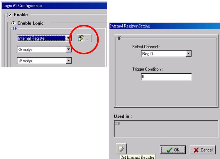
In the above figure, the "Used in:" column indicates that this Internal Register is also used with Rule-0, which helps the user identify the relationship between the rules. Also, the Set Internal Register button (
