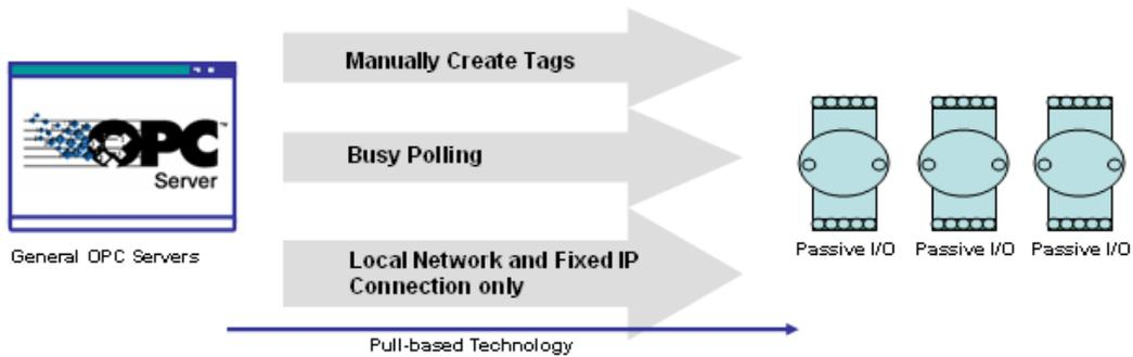
Moxa’s ioLogik Active Ethernet I/O products offer I/O status reports via TCP/UDP messaging, e-mail, and SNMP traps. In addition, they now support OPC technology. An ioLogik can automatically generate tags without requesting any data or even a device’s IP address. All the user needs to do is launch the Active OPC Server program, and the I/O channels selected by the user will be “pushed” from the ioLogik to the Active OPC Server.
