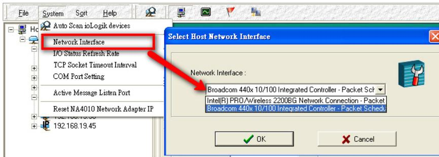
**NOTE** If multiple ioLogik W5300 units with same default IP address are installed on the same network, you will need to assign a different IP address to each unit to avoid IP conflicts. ioAdmin automatically detects IP conflicts and gives you a chance to modify each unit’s IP address in the **IP Address** column. Click the **Set** button to reboot the corresponding unit with its new IP address. Click the **Re-Search** button to refresh the list of units found by ioAdmin.
