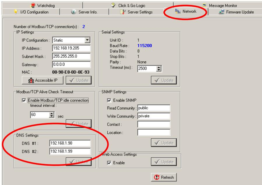
**Note: The DNS is required for both GPRS communication and a wired Ethernet LAN.**
