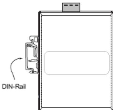
To remove ioLogik W5300 from the DIN-Rail, insert a flat-blade screw driver horizontally into the DIN-Rail kit under the ioLogik, and then pry it upwards to release the ioLogik W5300 towards and you away from the DIN-Rail.
