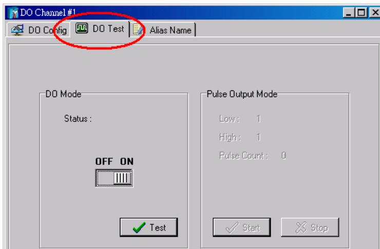
Use the Test panel to see how a channel’s status affects or is affected by the attached device. For DO/Relay Output channels, you can set the on/off status or start and stop pulse output. For DI channels, you can monitor the attached device’s on/off status, or monitor the counter.
