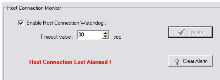
After you restore the network connection, click **Clear Alarm** to reset the Watchdog and return to normal operation.
