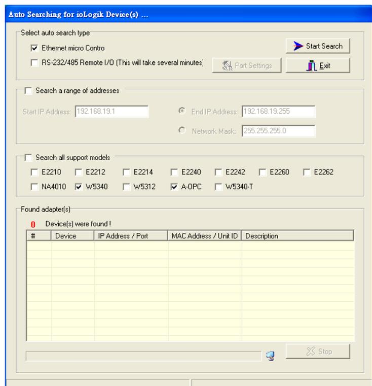
The auto scan function allows you to search for ioLogik devices automatically. You can search for these devices by type, IP range, or model name.
