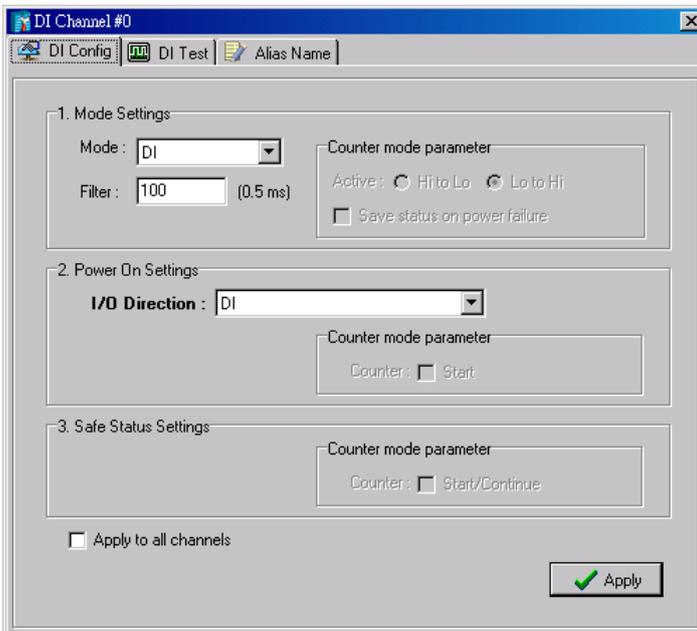
A DI channel can be set to "DI" or "Event Counter" mode. In DI mode, the specifications are as follows:
