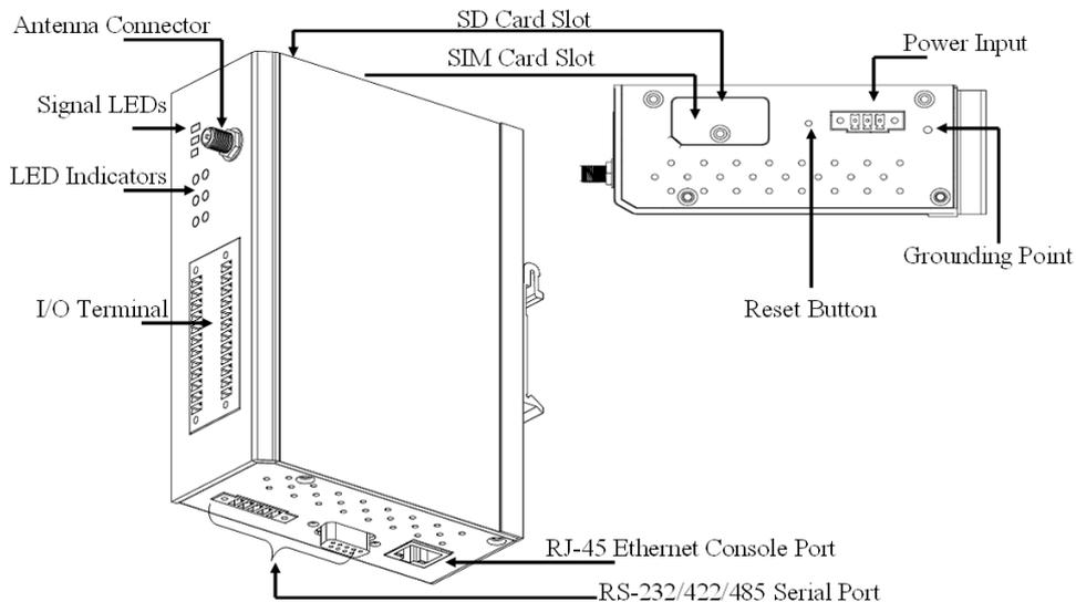
**NOTE** The reset button restarts the server and resets all settings to factory defaults. Use a pointed object such as a straightened paper clip to hold the reset button down for 5 sec. The RDY LED will turn red as you are holding the reset button down. The factory defaults will be loaded once the RDY LED turns green again. You may then release the reset button.
