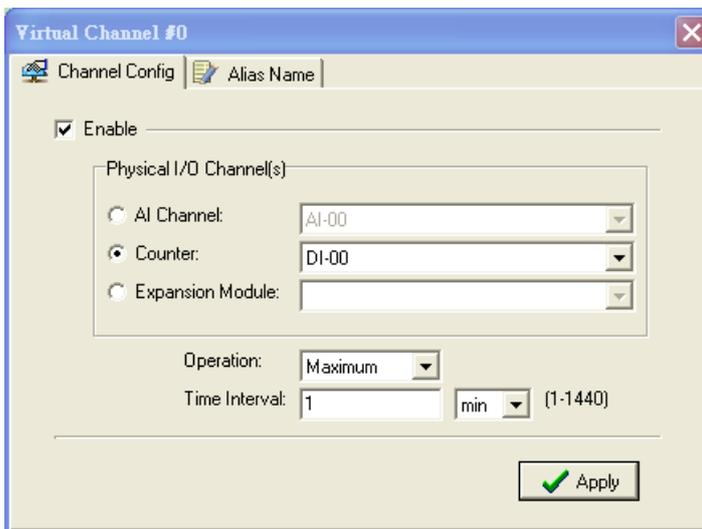
Next, choose the statistics function and time interval. There are six functions: Max, Min, Average, Accumulation, Instantaneous, and Incremental. The time unit can be set to minutes or hours, with a maximum value of 1440.
