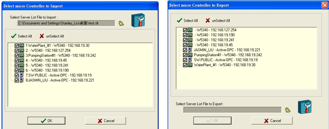
The file will have an .SLT extension and can be opened as a text file. The server list will provide the basic information for each server, such as **Device Name**, **Model**, **IP address**, and **Unit ID**.
