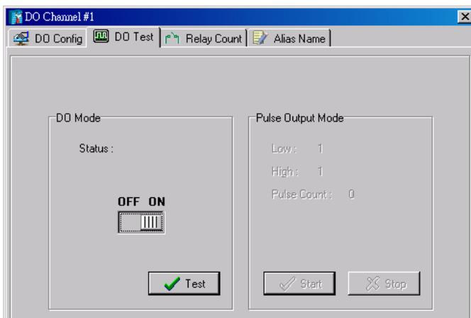
The Test panel shows how a channel’s status affects, or is affected by, the attached device. For output channels, you can set the on/off status, start and stop a pulse, or output a voltage or current. For input channels, you can monitor the attached device’s on/off status, counter, or input voltage/current.
