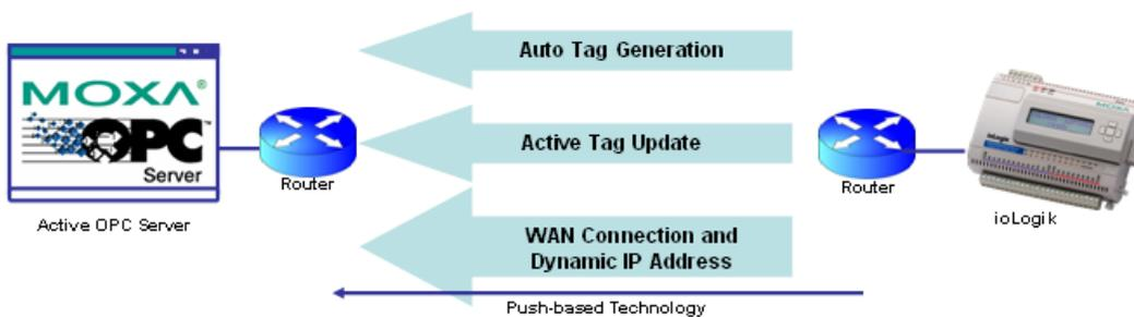
The “push” technology also includes the update for the tags. When the I/O status changes, the ioLogik will send updates to the Active OPC Server Lite. Compared to polling the status (the so-called pull-based method), this feature efficiently reduces network bandwidth usage and speeds up response time with event-driven, push-based status updates. At the same time, the heartbeat function monitors the system’s basic signs of life.
