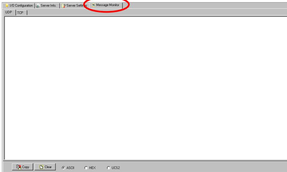
Messages can be displayed in ASCII, HEX or UCS2. To display messages in HEX, make sure the "HEX" button at the bottom of the window is checked. UCS2 stands for "Unicode System," which supports multiple languages.
