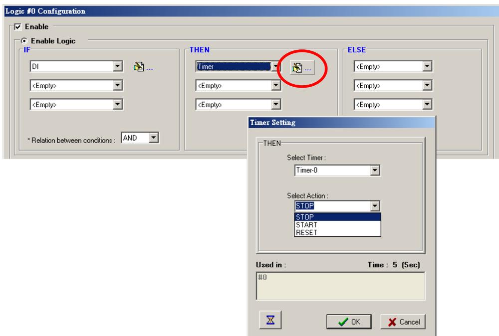
In the above figure, the "Used in:" column indicates this Timer is also used in Rule-0, which helps the user
