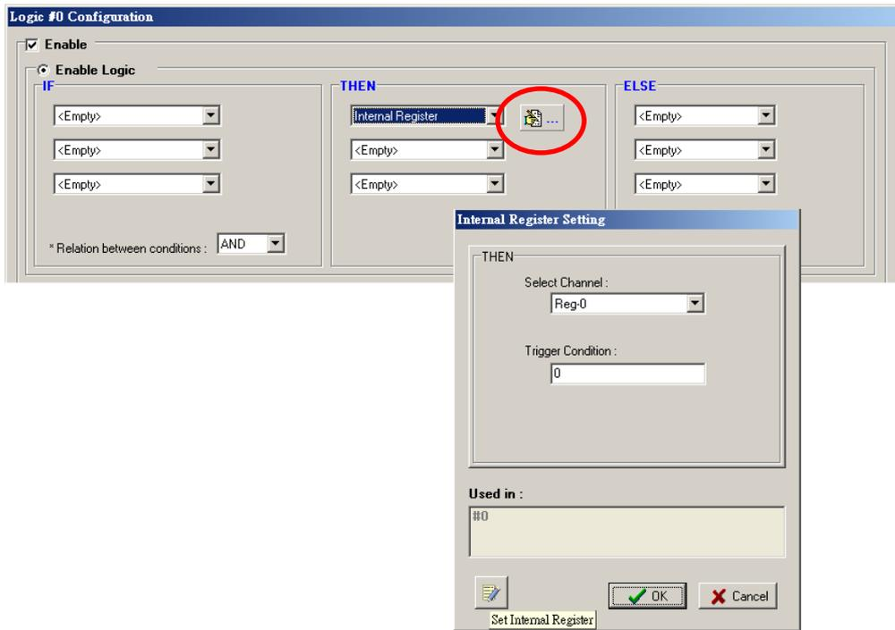
In the above figure, the “Used in:” column indicates that this Internal Register is also used in Rule-0, which helps the user identify the relationship between the rules. In addition, the Set Internal Register button (
