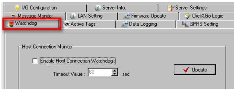
After the Watchdog is enabled, a warning will be displayed on the Watchdog panel if the network connection is lost.
