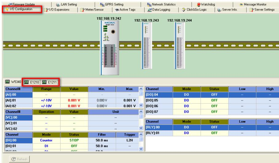
Double-click the expansion I/O tab (for example, for the E1210) to check the I/O status and set the alias name of the selected I/O channel.
