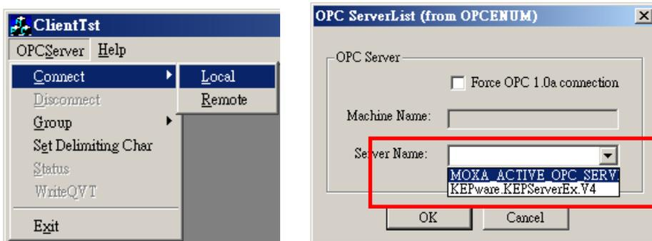
If Active OPC Server Lite is installed in a remote PC, select **Connect** → **Remote** from the menu bar. Input the host name (e.g.l, Moxa\_Client) or IP address and specify **MOXA ACTIVE OPC SERVER** in the **Server Name** column.
