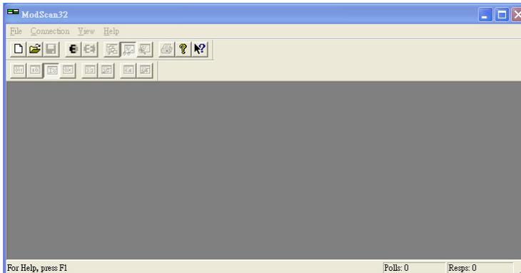
**Step 8:** Click **Connection** on the toolbar and choose **Remote TCP/IP server** in the **Connect Using** column. Input the W5300's IP address in the **IP Address** column and then click **OK**.
