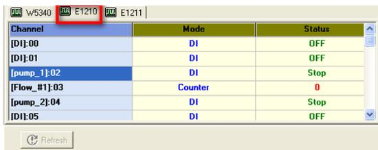
Note that you cannot configure the expansion module’s operation mode with ioAdmin. The configuration must be done with the E1200 configuration tool.
