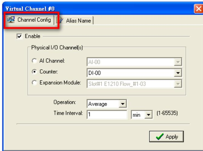
**Step 8:** Select the operation mode from Max, Min., Average, Accumulation, Instantaneous, and Incremental.
