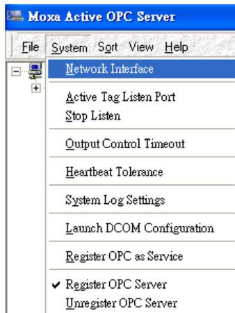
**Network Interface:** Select which network to use if the PC has multiple network adaptors installed.
