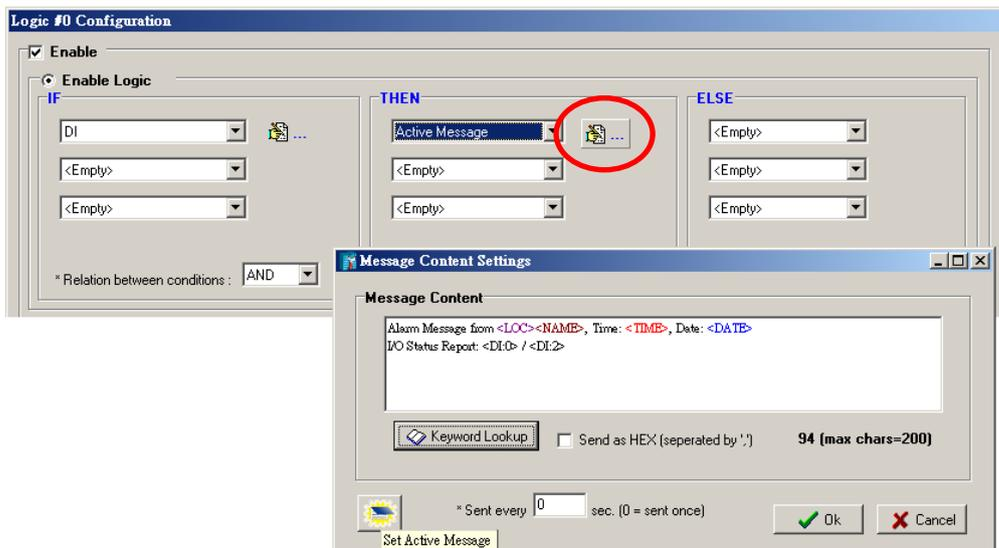
Active Messages can be received by a program using standard sockets, Moxa MXIO library, or ioAdmin’s Message Monitor, as shown in the following screen shot:
