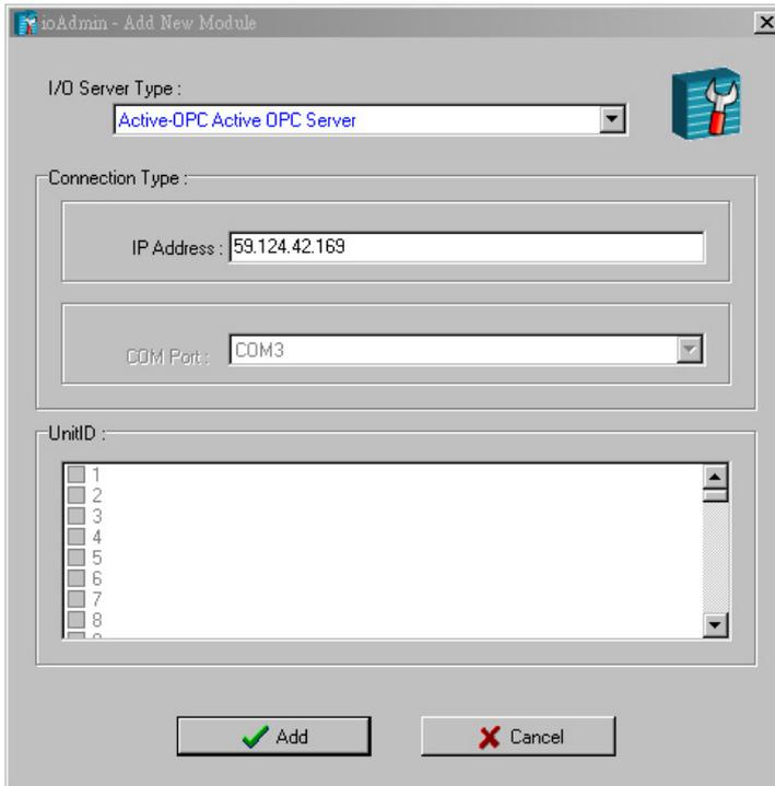
**Step 9:** After adding Active OPC Server you should see the following screen. Click the "Refresh" button to use ioAdmin to monitor and configure the ioLogik W5340.
