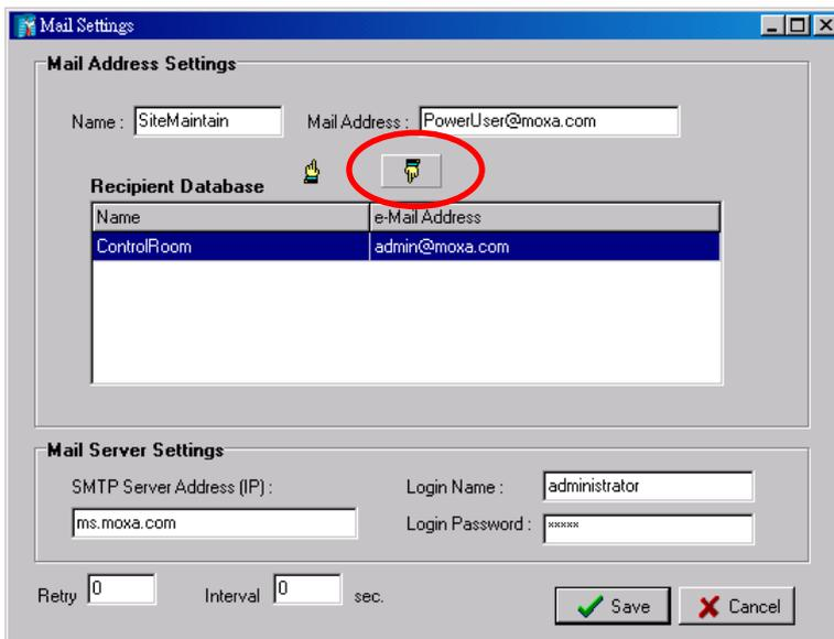
Under Mail Server Settings, you must configure the address of the SMTP server with your username and password. When using an FQDN (Fully Qualified Domain Name) address, such as ms.moxa.com, you must specify the ioLogik’s DNS settings.
