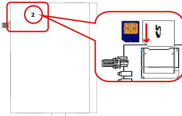
3. Open the card cover and insert the SIM/SD card. The card reader will release the SIM/SD card, after which you can pull the card out.
