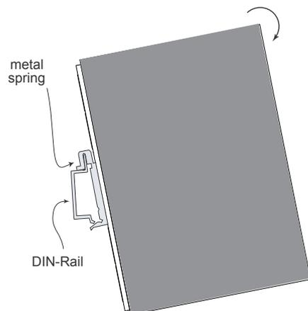
**STEP 2:** The DIN-Rail attachment unit will snap into place as shown.
