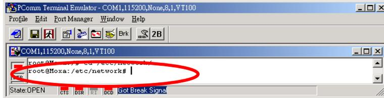
2. Type `#vi interfaces` to use vi editor to edit the network configuration file. You can configure the Ethernet ports of the IA3341 for **static** or **dynamic** (DHCP) IP addresses.
