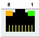
The UC-8416 has 8 10/100 Mbps switch ports. The LED indicators and pin assignments are exactly the same as the Ethernet ports.
