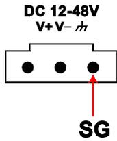
**SG:** The *Shielded Ground* (sometimes called *Protected Ground*) contact is the right most contact of the 3-pin power terminal block connector when viewed from the angle shown here. Connect the SG wire to an appropriate grounded metal surface.
