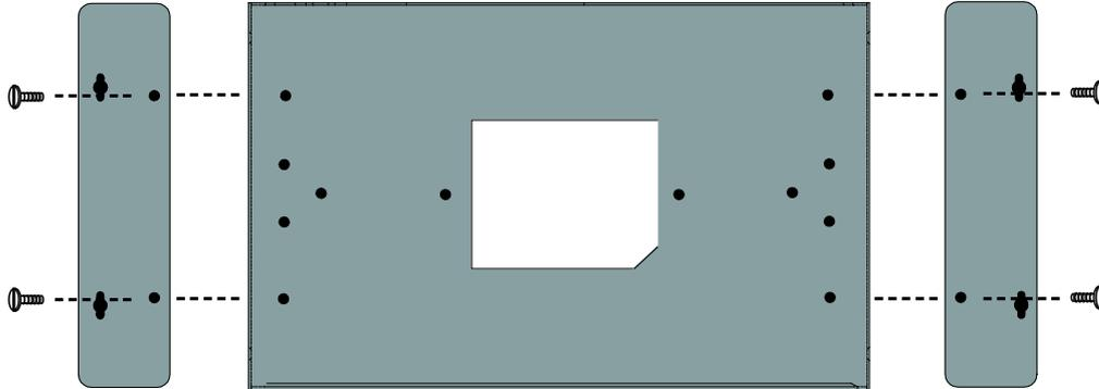
Figure A: UC-8410/8416/8418/8430 Embedded Computer—Wall Mounting Brackets (bottom view)
