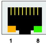
The lower right corner LED indicator maintains a solid green color when the cable is properly connected to a 100 Mbps Ethernet network. The LED will flash on and off when Ethernet packets are being transmitted or received.
