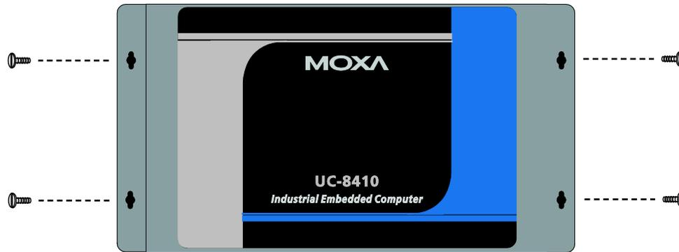
Figure B: UC-8410/8416/8418/8430 Embedded Computer—Wall Mounting Brackets (top view)
