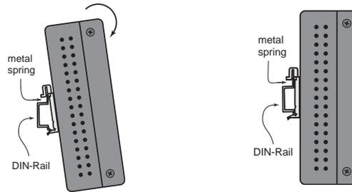
To remove UC-7402 from the DIN-Rail, simply reverse Steps 1 and 2 above.
