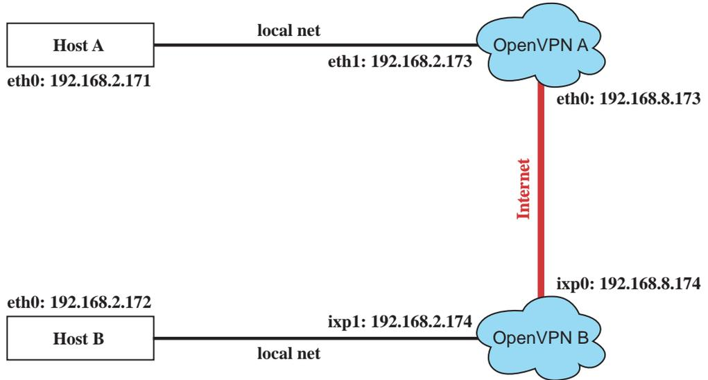
2. The configuration procedure is almost the same as for the previous example. The only difference is that you will need to comment out the parameter "up" in "/etc/openvpn/A-tap0-br.conf" and "/etc/openvpn/B-tap0-br.conf".
