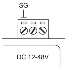
**SG:** The *Shielded Ground* (sometimes called *Protected Ground*) contact is the left most contact of the 3-pin power terminal block connector when viewed from the angle shown here. Connect the SG wire to an appropriate grounded metal surface.
