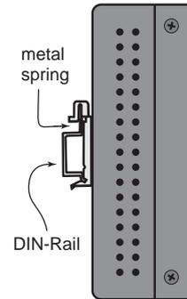
To remove UC-7420/7410 from the DIN-Rail, simply reverse Steps 1 and 2 above.
