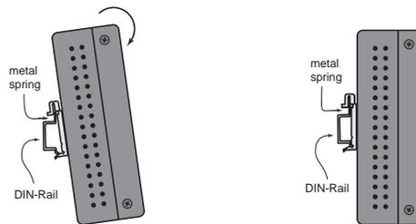
To remove UC-7420/7410 from the DIN-Rail, simply reverse Steps 1 and 2 above.
