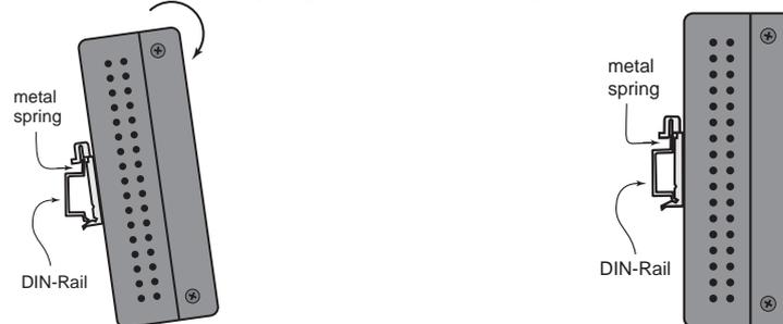
To remove UC-7408 from the DIN-Rail, simply reverse Steps 1 and 2 above.
