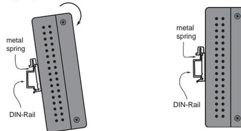
To remove the UC-7408-LX Plus from the DIN-Rail, simply reverse Steps 1 and 2 above.
