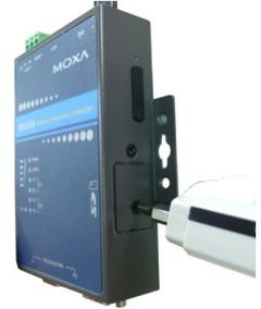
**Step3:** When inserting the SIM card, make sure the chip is facing upwards. Plug the SIM card directly into the slot.
