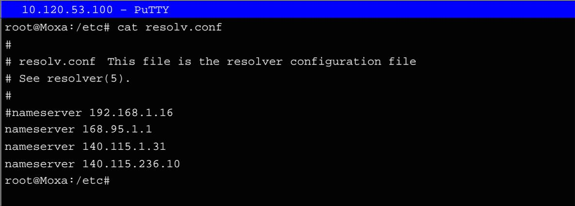
A terminal window titled "10.120.53.100 - PuTTY" showing the command "cat /etc/resolv.conf" and its output. The output lists several nameserver entries, with the first one being commented out with a hash symbol. The terminal background is black and the text is white.
