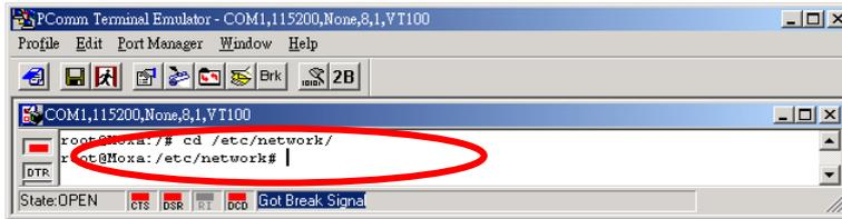
2. Type `#vi interfaces` to use vi editor to edit the network configuration file. You can configure the Ethernet ports of the W315A/325A for **dynamic** (DHCP) IP addresses.
