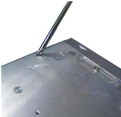
3. Grab hold of the main screw and lift to remove the V481's bottom cover. You will see that the socket is attached to the bottom cover.
