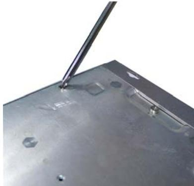
3. Grab hold of the main screw and lift to remove the V481's bottom cover.
