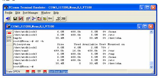
If there isn't enough "Available" space for your application, you will need to delete some existing files. To do this, connect your PC to the W315/325/345 with the console cable, and then use the console utility to delete the files from the W315/325/345's flash memory. To check the amount of free space available, look at the directories in the read/write directory /dev/mtdblock3. Note that the directories /home and /etc are both mounted in the directory /dev/mtdblock3.
