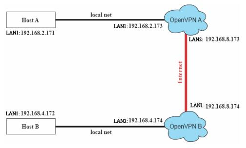
Host A (B) represents one of the machines that belongs to OpenVPN A (B). The two remote subnets are configured for a different range of IP addresses. When this setup is moved to a public network, the external interfaces of the OpenVPN machines should be configured for static IPs, or connect to another device (such as a firewall or DSL box) first.
