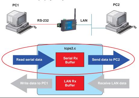
NOTE The **tcps2.c** application is a simple example designed to give users a basic understanding of the concepts involved in combining Ethernet communication and serial port communication. However, the example program has some limitations that make it unsuitable for real-life applications.
