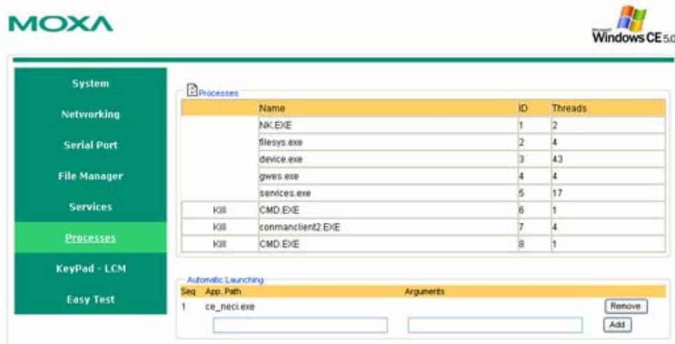
**Step 2.** In the first text field, enter the full path of the application. In the second text field, enter any arguments, if required. Click “Add”.
