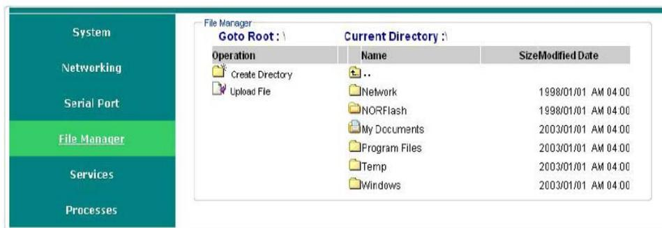
In addition, the management system offers a mechanism for file upload. This mechanism helps you transfer files from your workstation to the target computer in an easy way. For instance, after you have built an application on the development workstation, you can use this mechanism to upload the application to the current directory of the target computer.
