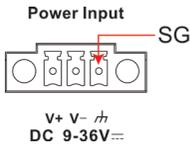
**SG:** The Shielded Ground (sometimes called Protected Ground) contact is the right most of the 3-pin power terminal block connector when viewed from the angle shown here. Connect the SG wire to an appropriate grounded metal surface.
