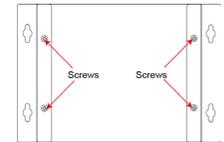
**STEP 2:** Use four screws per side to attach the V2101 to a wall or cabinet.
