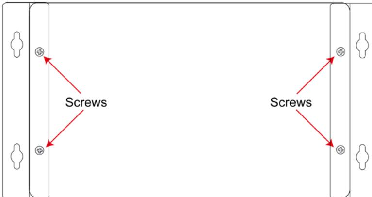
**Step 2:** Use two screws per side to attach the V2401/2402 to a wall or cabinet.
