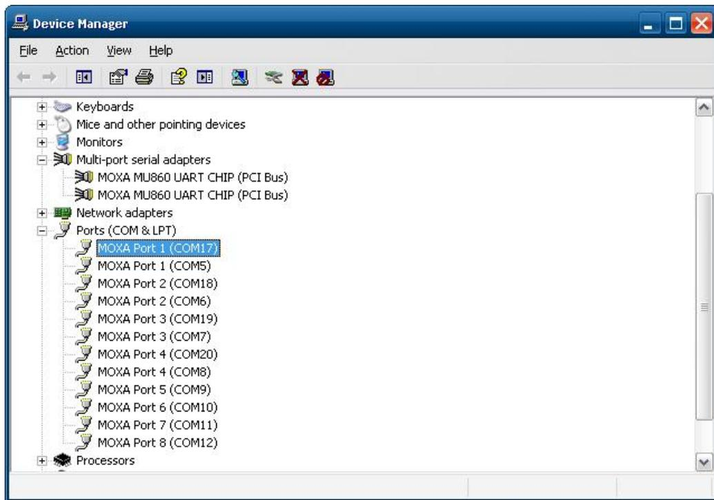
**NOTE:** Make sure each port name is unique, or the duplicate names will lead to inaccessible devices.
