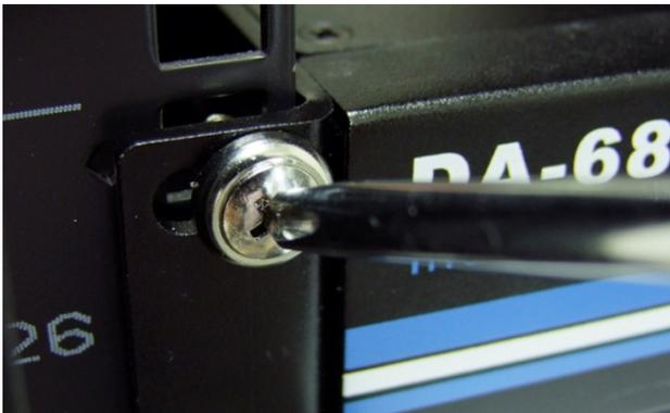
As a final check, make sure that the four screws are firmly attached to the rack.
