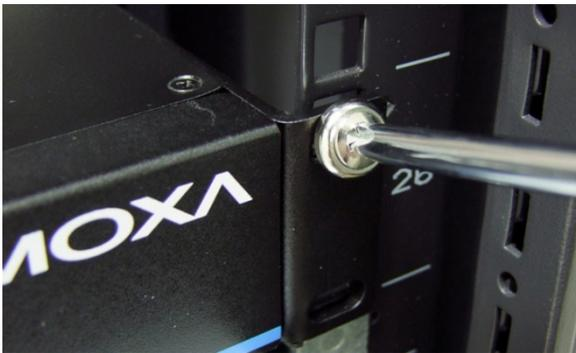
Note that four screws are required to attach the DA-681 to the rack. Use two screws on the left side and two screws on the right side.
