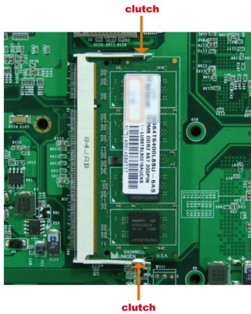
Gently insert the new memory into the module. Make sure the direction is correct.
