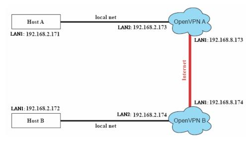
The configuration procedure is almost the same as for the previous example. The only difference is that you will need to comment out the parameter up in /etc/openvpn/tap0-br.conf of OpenVPN A and /etc/openvpn/tap0-br.conf of OpenVPN B.
