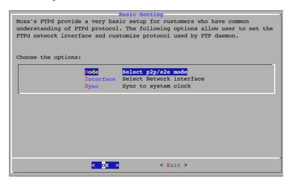
Select **P2P** (Peer-to-Peer) mode or **E2E** (End-to-End) mode for the PTP protocol. When finished, select **OK** to continue.
