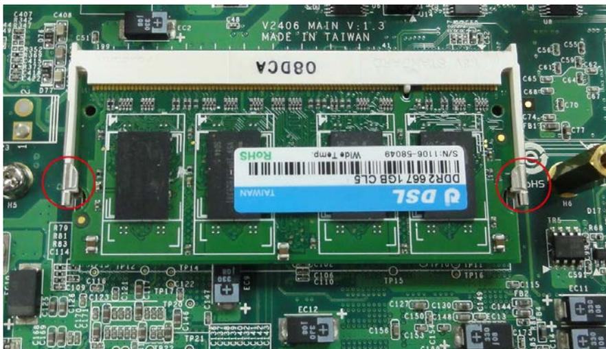
6. Push down the module and make sure the latches are firmly in place.
