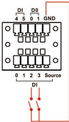
**DI Wet Contact Wiring**
