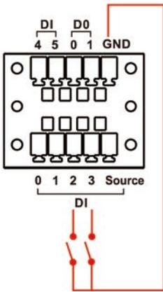
**DI Wet Contact Wiring**
