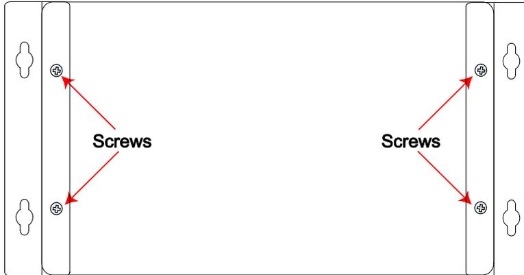
**Step 2:** Use two screws per side to attach the V2406-24I to a wall or cabinet.
