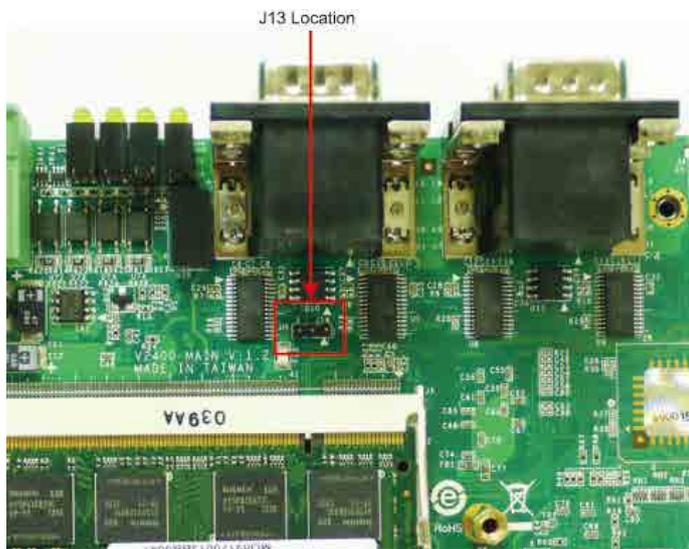
Use the jumper to select the voltage for PIN 9 of the Serial Port 1. Refer to the following table for jumper settings.
