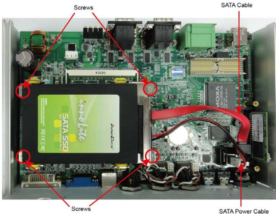
9. Connect the SATA power cable and the SATA cable to the connectors.
