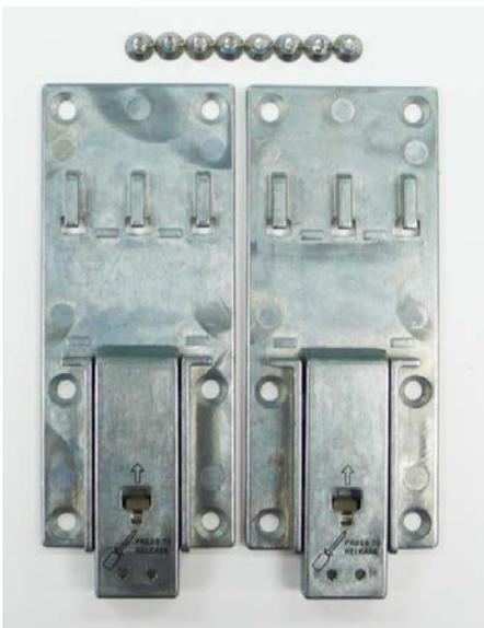
To attach the DIN-rail kit, turn the V2406-24I over to the bottom cover. Find the locations for the screws and place the brackets on the cover. Please note that all eight screws must be firmly attached so that the computer can be securely installed on the DIN-rail.
