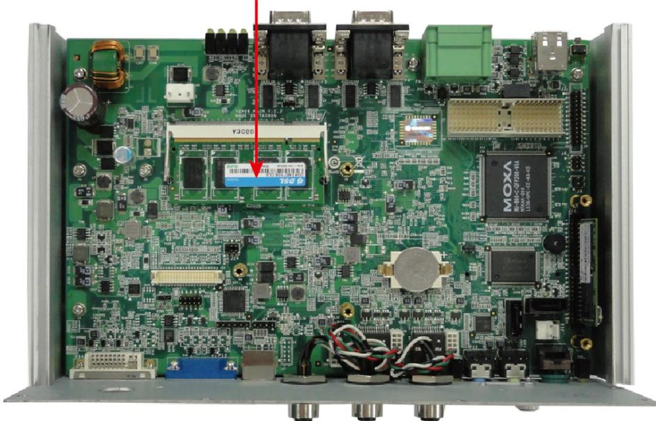
5. Carefully remove the module by pushing the latches on both sides of the module, and then replace the new module. Be sure to orient the module correctly.
