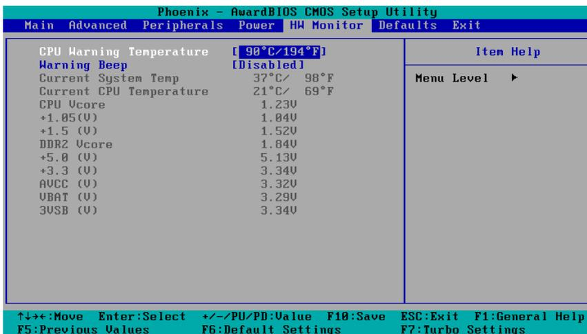
This item helps monitor the status of the system, including CPU temperature and the voltage of the CPU, SDRAM and battery.
