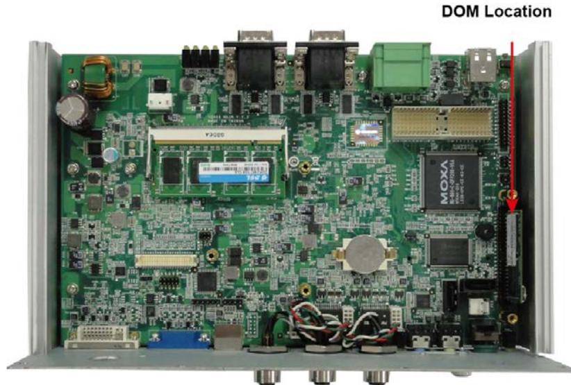
2. Pull up and take off the DOM module, and then place the new DOM module into the slot.
