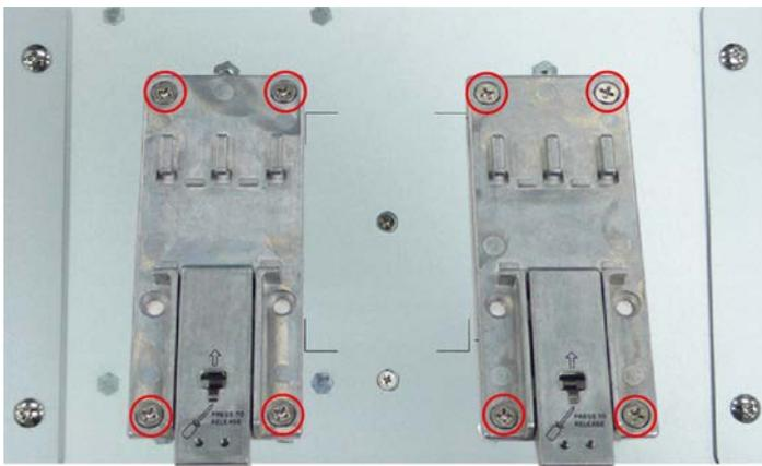
When the brackets are firmly attached with the screws, it can be installed on a DIN-rail
