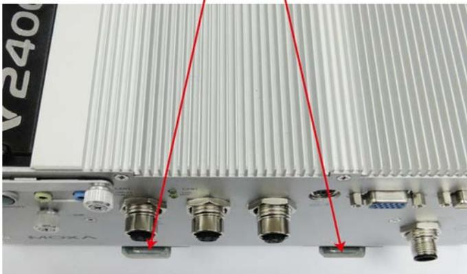
To re-install the computer on the DIN-rail, use a screwdriver to press the buckle so that it can be released. Now, it can be re-installed on the DIN-rail.
