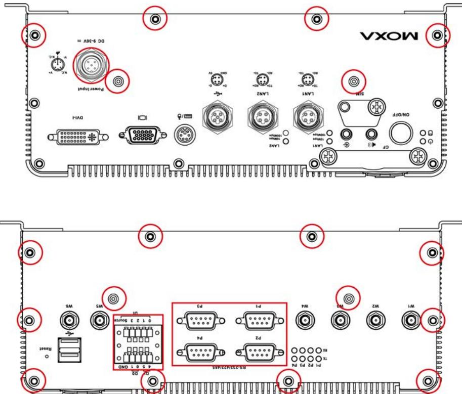
3. Remove the cover of the rear panel, and disconnect the internal power connector.
