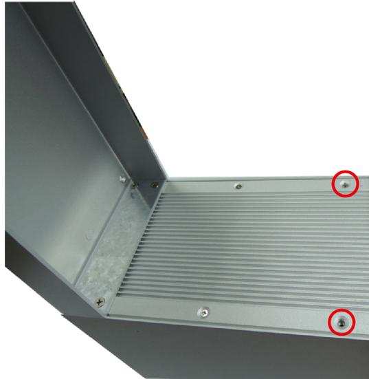
**Step 4:** Place the support panel so that it abuts the extension panel, with the screw holes aligning with the two flanges on both the panel and the right corner of the computer. Place the toothed locking washer over the screw holes on the computer's right side, then use the dome headed screws to fasten the support panel to the side of the computer.
