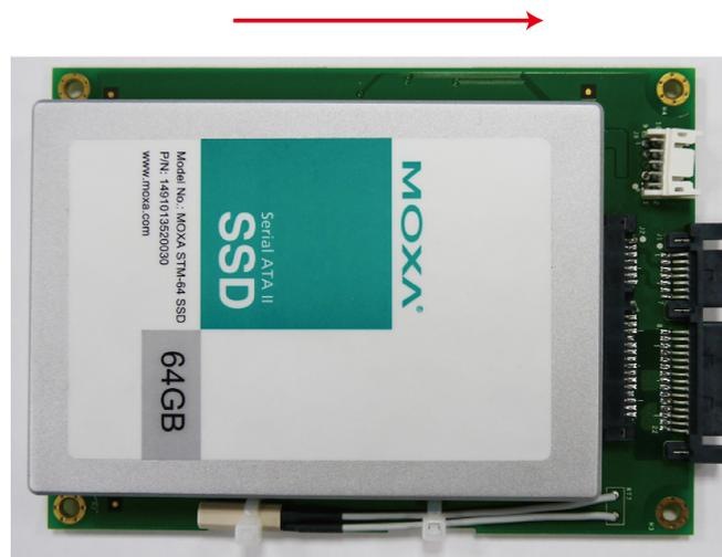
**Step 6:** Turn back the tray and fasten the drive to the PCB using the holes indicated below.
