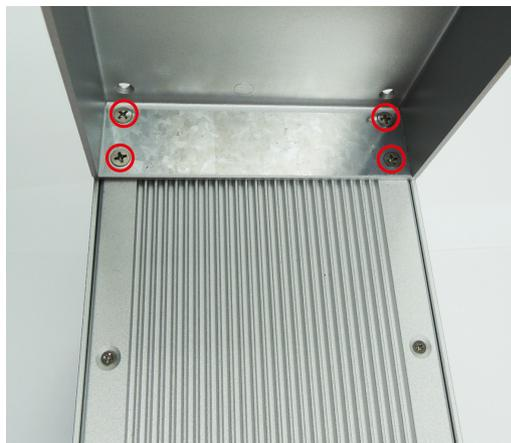
**Step 3:** Remove the two rear-most screws from the right side of the computer.
