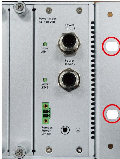
After installing the rack mounting assembly (handles and/or ears), four screws are required to fasten the TC-6110 to a rack.
