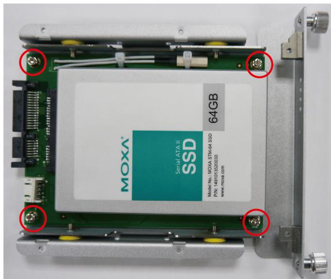
**Step 8:** Connect the power cable and SSD/HDD cable with the main board. Reconnect the data and power interfaces and complete the installation by fastening the drive tray to the main PCB using the six screws.
