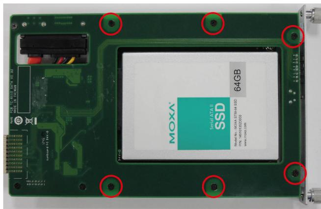
**Step 9:** When finished, insert the storage tray back into the TC-6110 and tighten the external thumbscrews.
