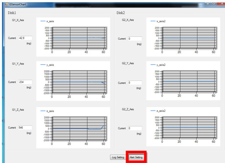
2. When the **AlertSetting** interface appears, it will look like the screenshot below. Generally, for industrial hard drives built with high tolerance for vibration and shock, a good point to begin with is 1000 mG (1 G)
