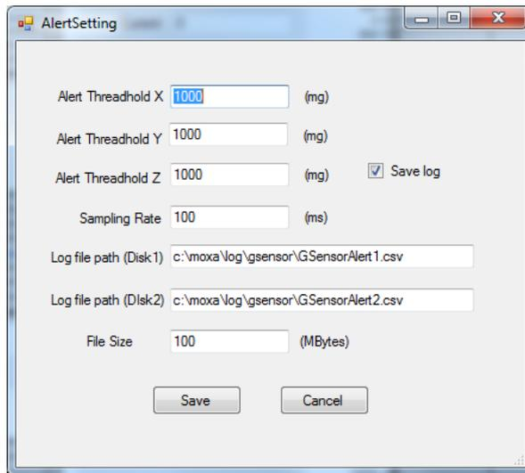
3. Click **Save** to finish the setup. **Note: Disk1 refers to slot 1, and Disk2 to slot 2.**
