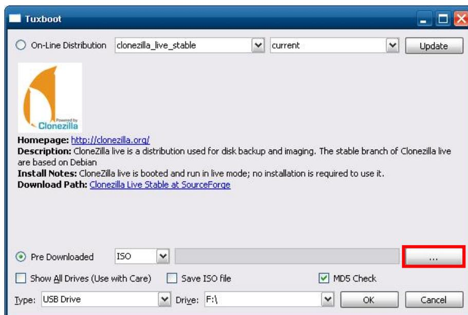
2. Navigate to `\recovery\TC6110W7E\ClonezillaFactory_2013-02-21-14\` on the software DVD and select the boot environment's ISO image.
