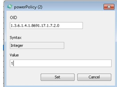
3. The **Set Value** dialog for the **powerPolicy** OID has two variable fields: one showing the OID that is being called and a second called **Value**, to indicate which power management policy should be used. Use the integer 1 to indicate the **Balanced**, 2 for the **Power Saver**, and 3 for the **High Performance** policy. After entering the value, close the dialog by clicking **Set**.
