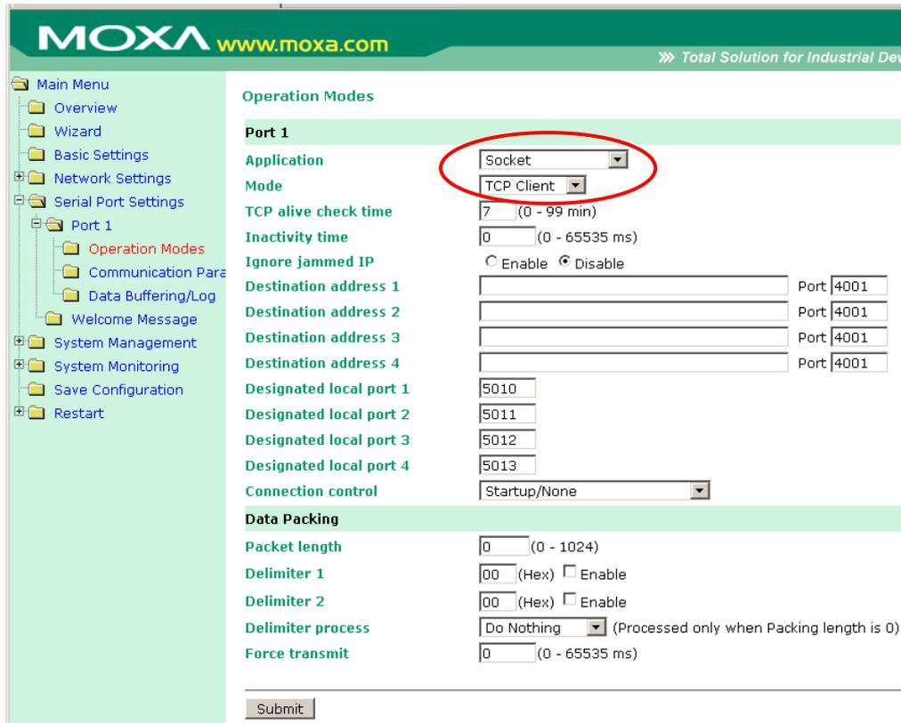
When **Mode** is set to **TCP Client** on a serial port's **Operation Modes** page, you will be able to configure additional settings such as **TCP alive check time**, **Inactivity time**, and **Ignore jammed IP**.
