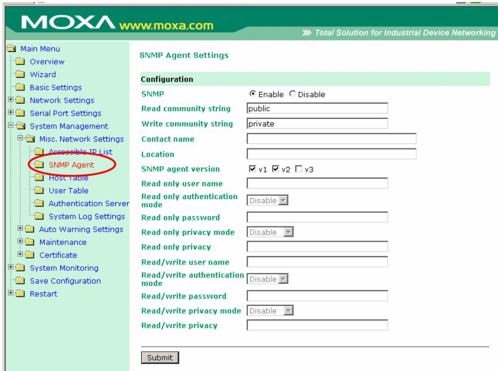
The **SNMP Agent** page is located under **Misc. Network Settings** in the **System Management** folder. This page is used to configure the SNMP Agent on the NPort.
