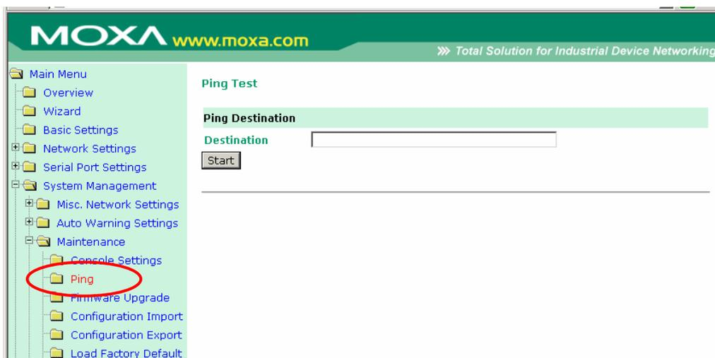
The **Ping** page is located under **Maintenance** in the **System Management** folder. It provides a convenient way to test an Ethernet connection or verify an IP address. Enter the IP address or domain name in the Destination field and click **[Start]**. The results will be displayed immediately.
