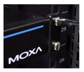
**NOTE** That four screws are required to attach the SMG-6100 to the rack. Use two screws on the left side and two screws on the right side.
