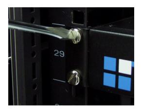
As a final check, make sure that the four screws are firmly attached to the rack.
