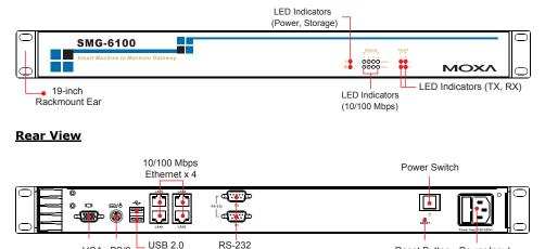
VGA PS/2 USB 2.0 RS-232 Host x 2 Serial Port x 2, DB9
