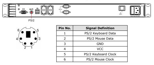
Use the Y-type cable to convert the mini-DIN connector into two 6-pin mini-DIN connectors to connect both a PS/2 keyboard and PS/2 mouse at the same time. (The Y-type cable is not included in the accessory package. It should be purchased separately. You may also use the USB ports to connect your USB-based keyboard and mouse.)
