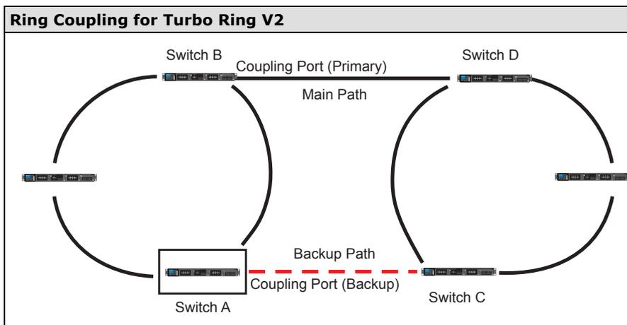
Note that the ring coupling settings for a **Turbo Ring V2** are different from a **Turbo Ring**. For Turbo Ring V2, ring coupling is enabled by configuring the **Coupling Port (Primary)** on Switch B and the **Coupling Port (Backup)** on Switch A only. You do not need to set up a coupling control port, so **Turbo Ring V2** does not require a coupling control line.
