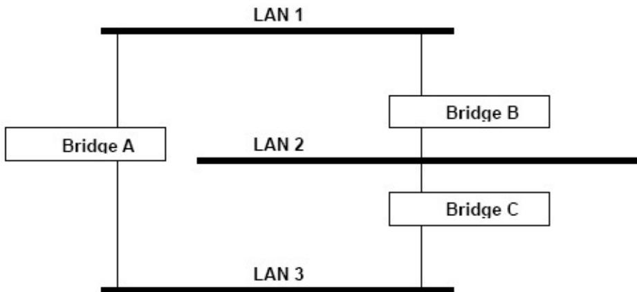
If STP is enabled, it will detect duplicate paths and prevent, or block, one of them from forwarding traffic. In the following example, STP determined that traffic from LAN segment 2 to LAN segment 1 should flow through Bridges C and A because this path has a greater bandwidth and is therefore more efficient.
