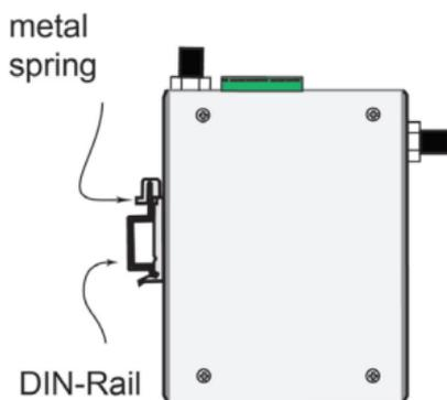
To remove the AWK-1127 from the DIN rail, simply reverse Steps 1 and 2.
