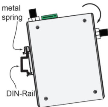
**STEP 2:** The DIN-rail attachment unit will snap into place as shown below.
