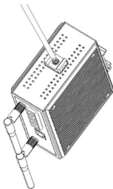
**STEP 1:** Screw the cable holder onto the bottom of the AWK-3121-SSC.
