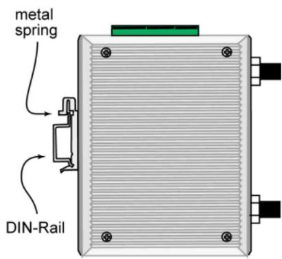
To remove the AWK-3121-SSC from the DIN-Rail, simply reverse Steps 1 and 2.
