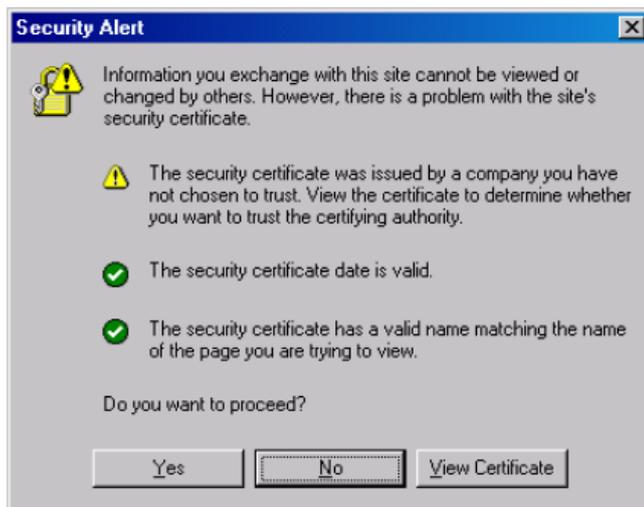
3. Select **Yes** to accept the certificate issued by Moxa IW and then enter the AWK-3121-M12-RTG's web browser interface secured via HTTPS/SSL. (You can see the protocol in URL is **https**.) Then you can use the menu tree on the left side of the window to open the function pages to access each of AWK-3121-M12-RTG's functions.
